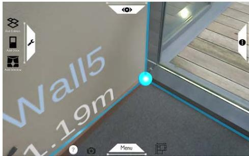
(a) *Freeze-Set-Go* interaction proposed by Easy Build to accurately position the room corners. Image courtesy of Wosomtech.
