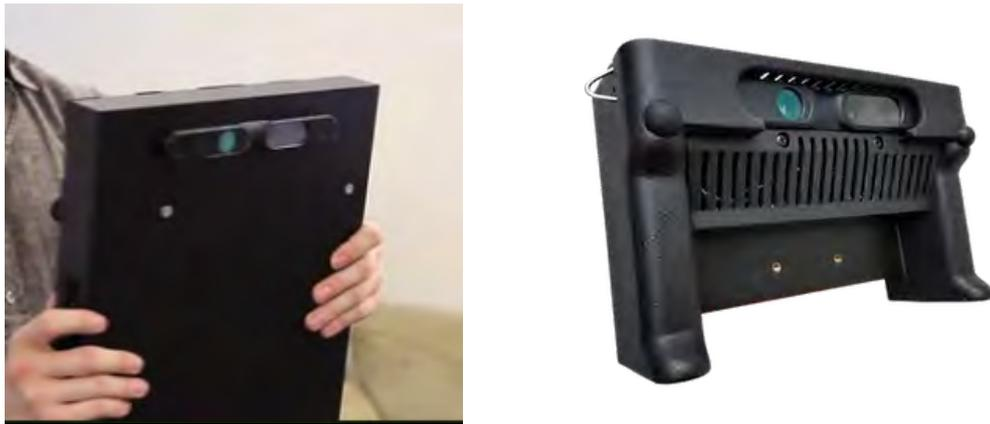
**Figure 4.2:** Desktop range imaging sensors fixed on tablets. On the left: Lynx Laboratories tablet. On the right, DOT Product DPI-8X.
