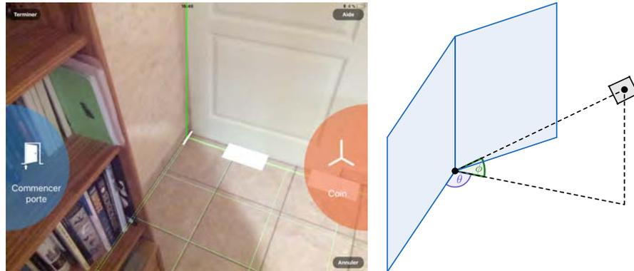
**Figure 5.1:** Selection of a 3D point with a crosshair with Magic Plan, the user has to adjust two rotations:  $\theta$  and  $\phi$ .
