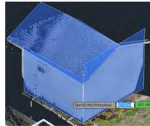
(c) Plane fitting on a point cloud with Revit. Image courtesy of Autodesk.
