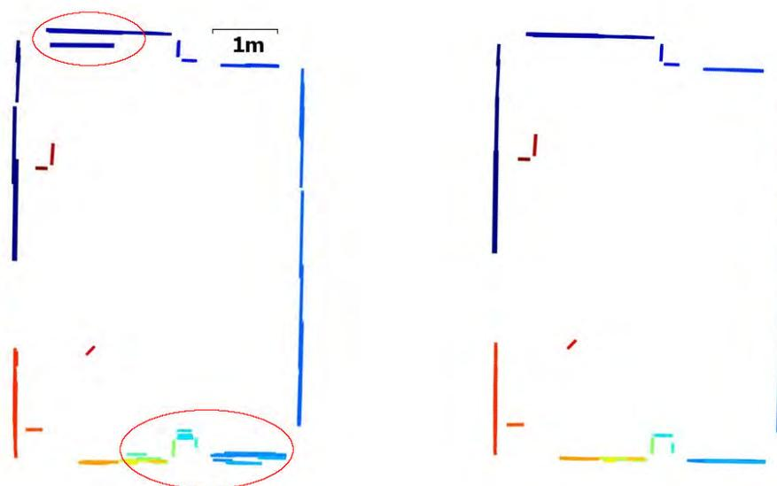
**Figure 4.31:** Left: initial planar uncertainty rectangles. Two uncertainty boxes are displayed with the same color if there are associated with the same fused-**PP**. The red ellipsis illustrates the regions where the odometry drift caused a notable duplication of the wall structure. Right: *uncertainty boxes* (defined in Figure 4.29b) drawn after the correction from our planar **LS SLAM**. To illustrate the enhancement of our method, we had disabled the **Tango** global map optimization.
