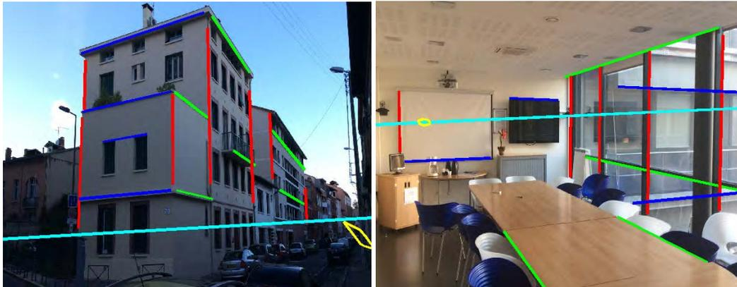
**Figure 3.14:** Some photos of the dataset with their ground truth line segments (red, green, blue), the horizon line computed from the IMU data (cyan line) and the polygon of the uncertainty region computed on the red line segments. In the photo on the left, the horizon line computed with the IMU data does not intersect the yellow polygons because of the bias of the IMU data.
