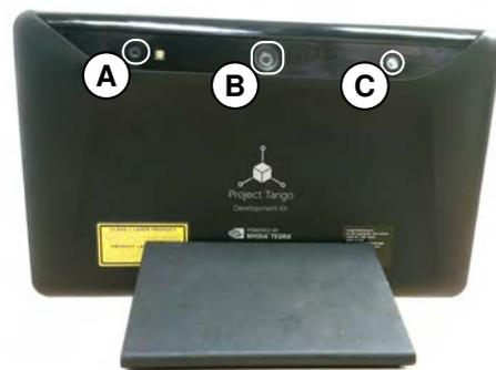
(b) Tango TDK image sensors – RGB-IR camera (A), Fisheye camera (B), IR pattern emitter (C).
