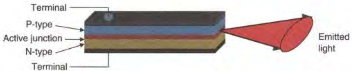
Fig. 1-18 Structure of the LED [52]
