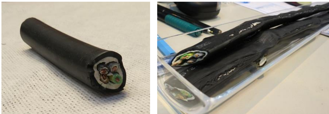
Figure 32: Flame retardant non-corrosive (FRNC) power cable sample (left), pressed cable sample (right).
