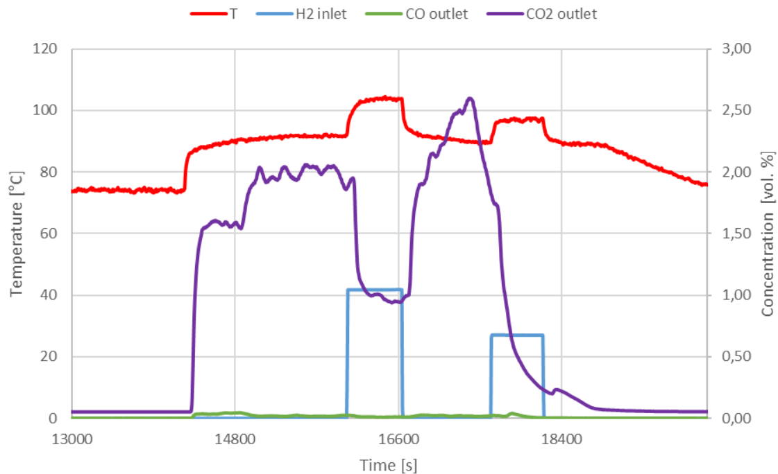
Figure 66: Pt catalyst behavior during well-ventilated combustion (RF-A-07)
