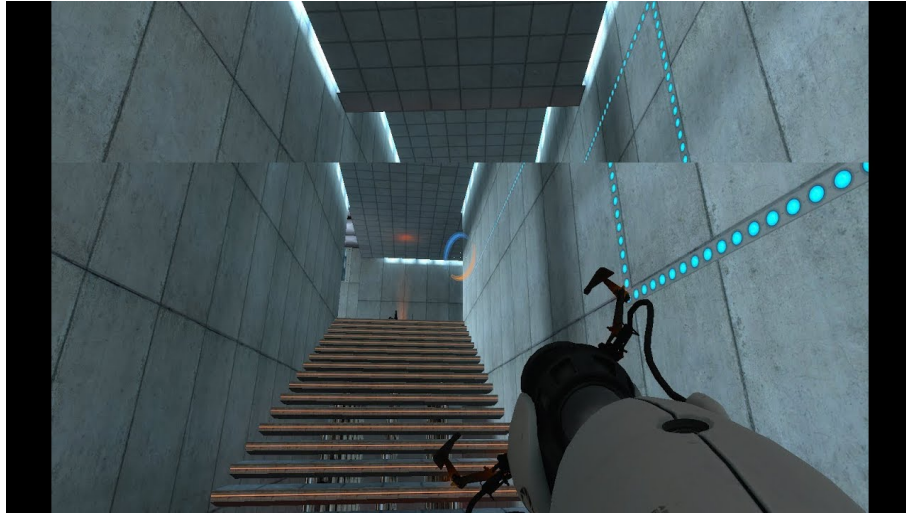
Figure 1.18: Example of Tearing in Portal (2007)
