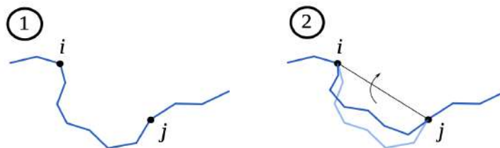
FIGURE A.4: Crankshaft move: Pick a random block of cylinders [i, j] . Rotate the block around the axis connecting the ends of the block by a random angle. (picture from (Lepage and Junier, 2017))
