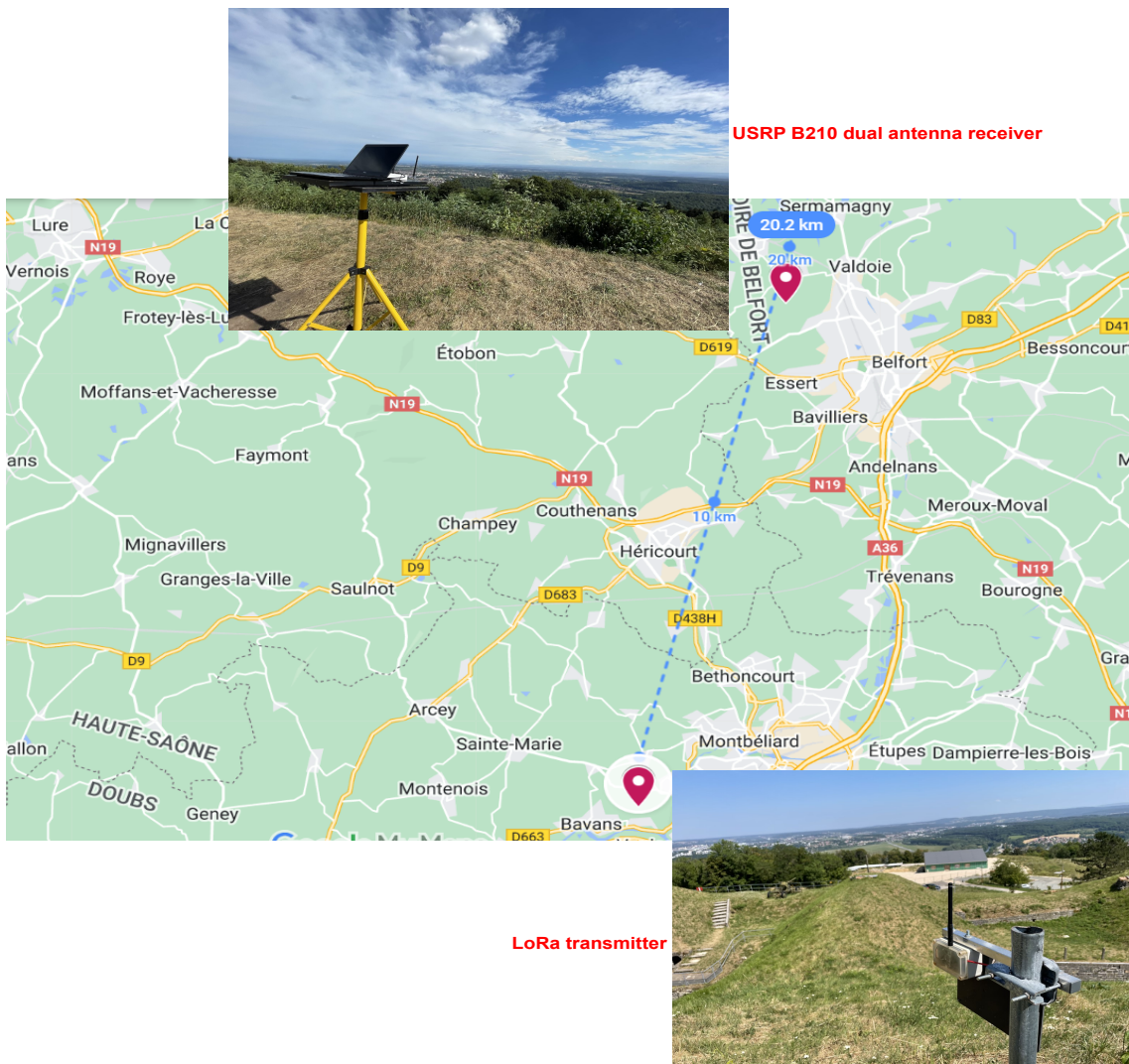
Figure 5.17: Google Maps image of our direction finding system in an outdoor environment with a distance of 20.2 km.
