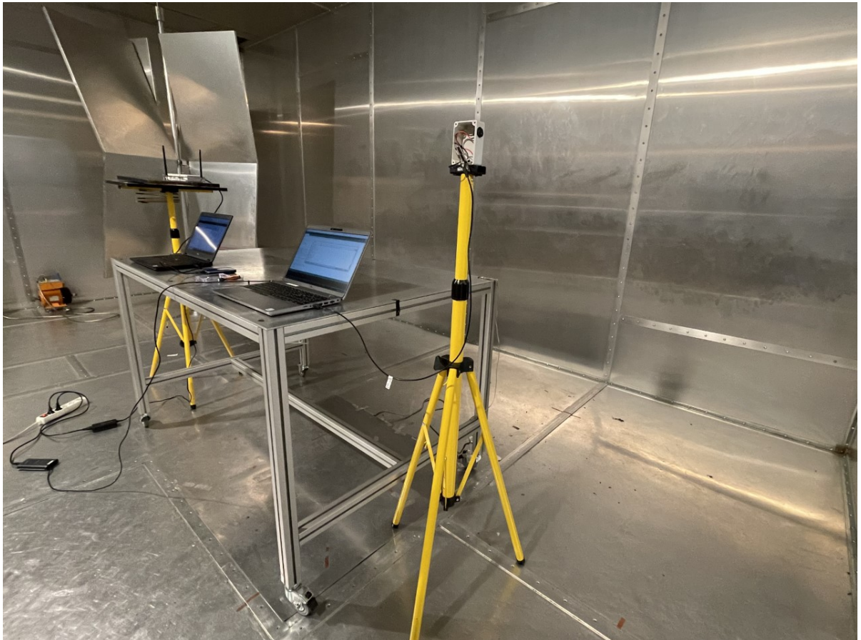
Figure 4.29: Experimental setup - two antennas direction finding system using USRP B210 and LoRa RFM95 in reverberation chamber.
