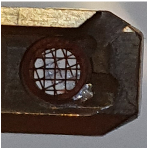
(a) Photo of the sample wedged between two grids and placed on a sample holder. The grids are 3 mm in diameter and are rotated with respect to each other. The sample is visible in between the grids.
