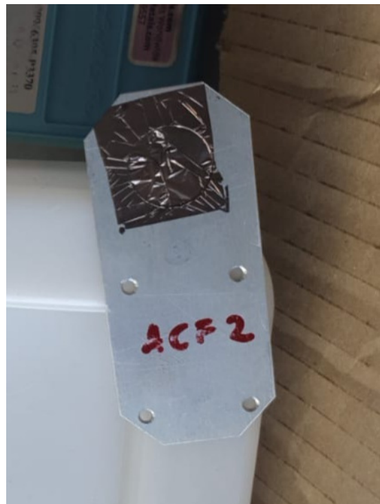
(d) Photo of an ACF Metal carbon foil deposited on the final support.
