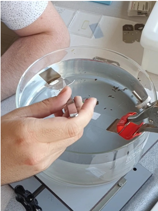
(c) Photo of an ACF Metal carbon foil being picked up with the final support.
