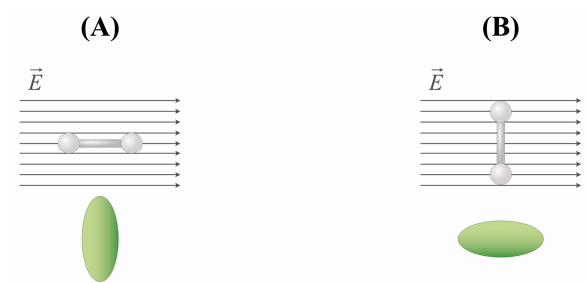
Figure 2.8: Hydrogen molecule (white balls with line as bond) in electric field with corresponding polarizability ellipsoid (green oval) below. (A) Hydrogen bond axis oriented parallel to electric field lines. (B) Bond axis oriented perpendicular to electric field lines.
