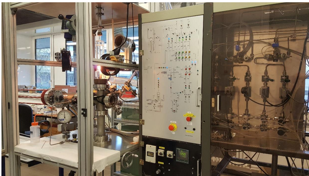
Figure VI.9: Home-made reactor used for SiC CVD growth in LMI facilities
