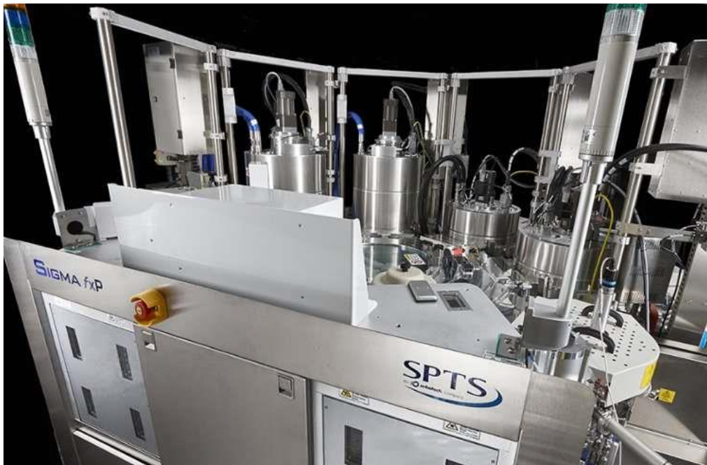
Figure III.12: SIGMA PVD equipment used for AlN PVD deposition 389
