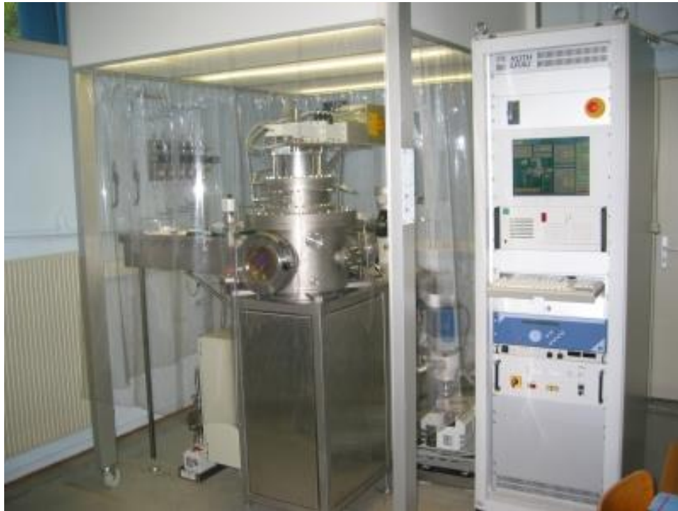
Figure 1: Photo of an electron cyclotron resonance - plasma enhanced chemical vapor deposition (ECR-PECVD) reactor.
