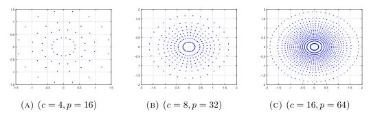
FIGURE 4.2: Three different GS-APSK.
