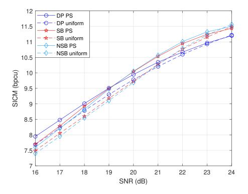
FIGURE 3.17: SICM performance of different schemes when using QAM signals.
