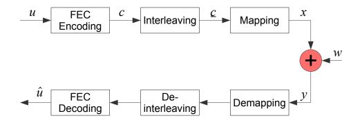
FIGURE 2.1: Simplified model of a coded transmission system over the additive Gaussian noise channel.
