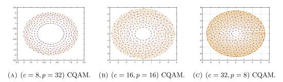
FIGURE 4.8: The different studied 256-CQAM constellation diagrams.
