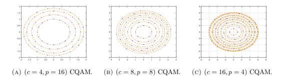
FIGURE 4.7: The different studied 64-CQAM constellation diagrams.
