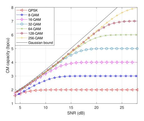
FIGURE 2.2: Capacity of uniform M-QAM formats.
