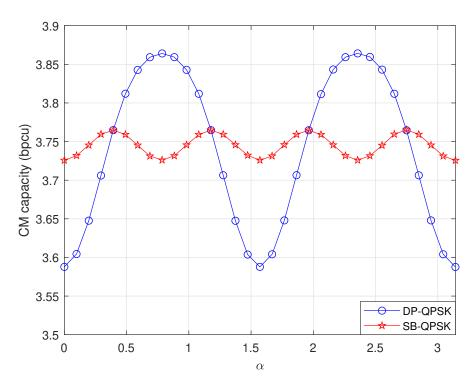
FIGURE 3.1: SB-QPSK rate as a function of  $\alpha$  at an SNR of 11 dB and for  $\Lambda = 6$  dB compared to the one of DP-QPSK.
