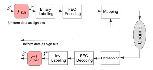
FIGURE 2.4: Block diagram of PAS.
