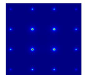
FIGURE 2.3: The constellation diagram of PS-16QAM.
