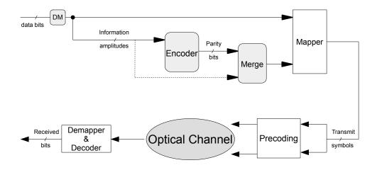
FIGURE 3.15: Optical communication system with binary PAS.
