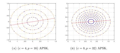
FIGURE 4.4: GS-APSK observed as rotated GS-PAM.
