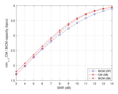
FIGURE 3.7: Worst CM and BICM rates for the SB and DP schemes as a function of SNR for  $\Lambda = 6$  dB.
