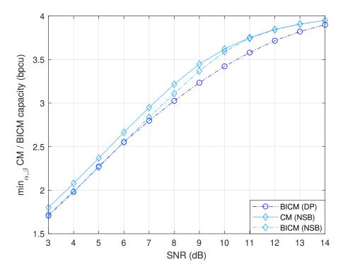
FIGURE 3.11: Worst CM and BICM rates for the NSB and DP schemes as a function of SNR for  $\Lambda = 6$  dB.
