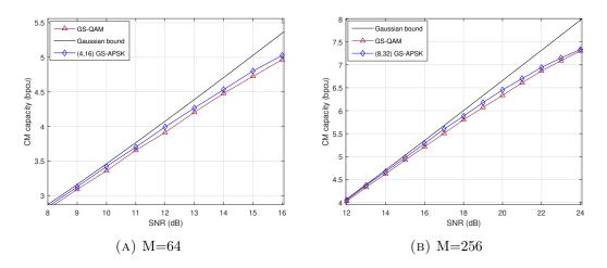
FIGURE 4.3: Comparison between the GS-QAM and GS-APSK
