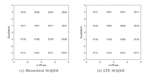
FIGURE 2.13: Examples of studied QAM constellation diagrams.
