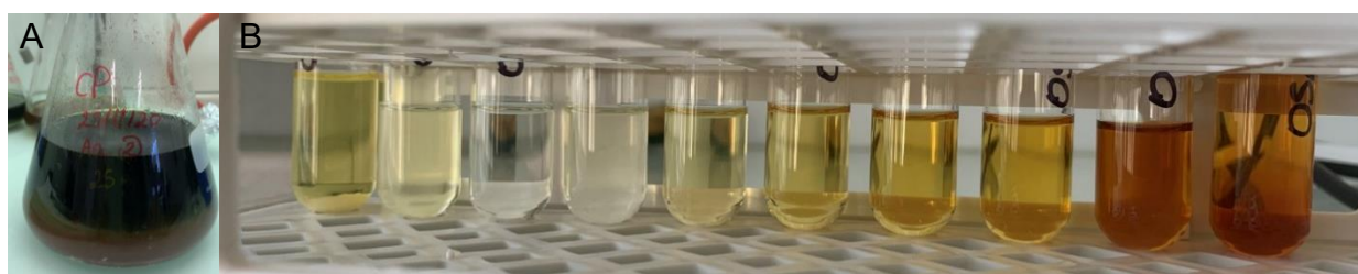
Figure 1: Macerate of algae powder in MeOH:DCM (A) and ten of the eleven fractions obtained after fractionation of the crude extract (B)
