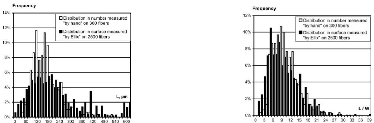
FIGURE 1.10: Comparison between "by hand" measurement and measurement made with a software for (a) fibers' length and (b) fibers' aspect ratio [8]
