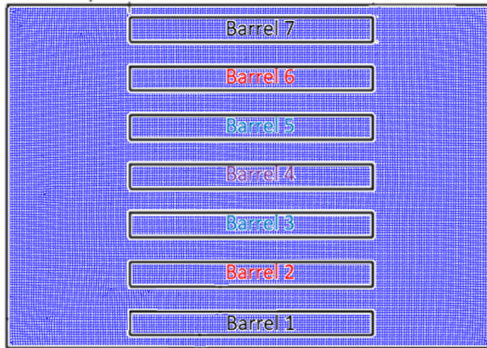
FIGURE 3.8: Mesh of the whole plate with barrels' location
