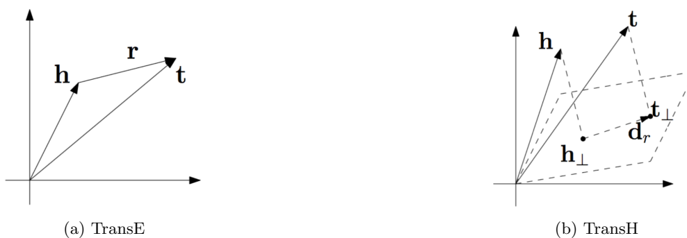
Figure 3.5: Visualizations of the TransE (a) and TransH (b) models. These figures are extracted from the original paper by Wang et al. [131].
