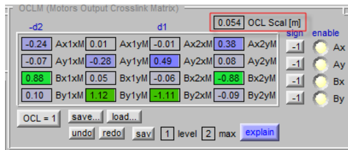
Figure 4.11: OCL matrix. Allows the decoupling of the four degrees of freedom. It defines the combination of movements of the four output actuators to achieve pure position or angle displacements.
