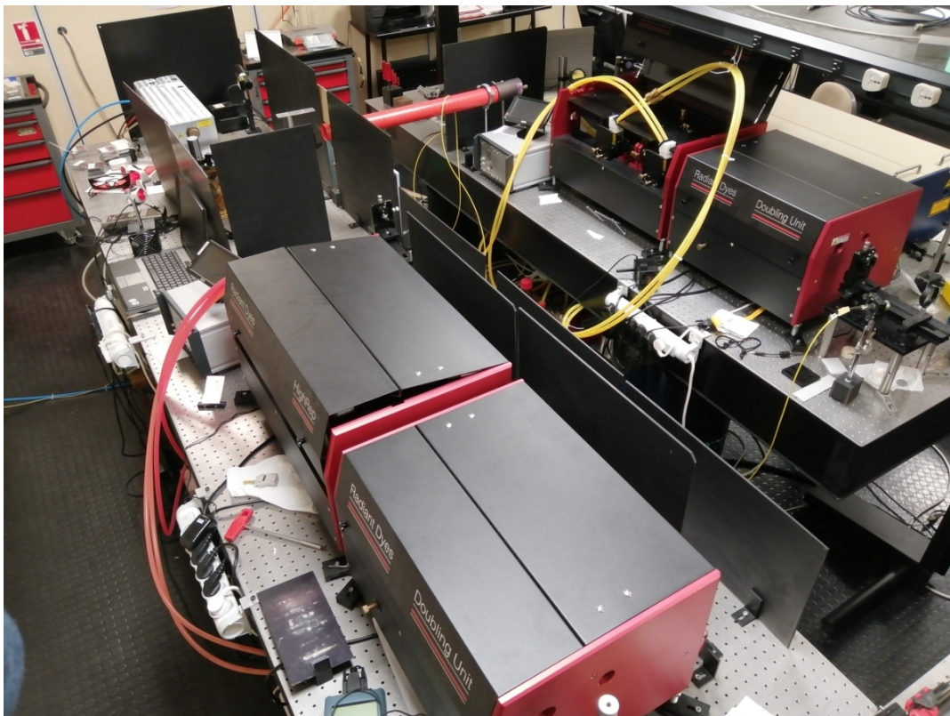
Figure 3.5: RIALTO laser system layout. Three tunable dye lasers pumped by a frequency double Nd:YAG laser.
