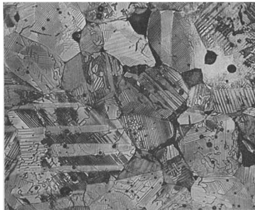
Figure 1.4: Microstructure of \text{BaTiO}_3 , a piezoelectric ceramic, after etching and polishing, showing its complex polycrystal structure. Picture obtained by a petrographic microscope using transmitted light [3]
