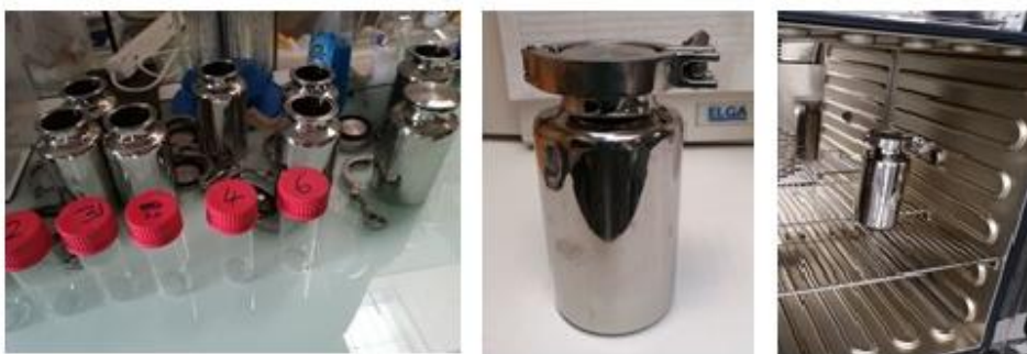
Figure 31: Original steel glass and steel bottles used for ageing in an oven.
