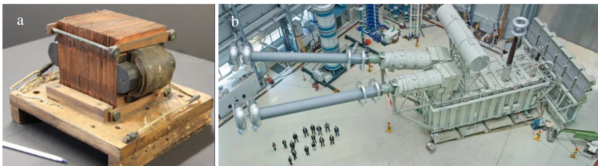
Figure 1: a: Picture of the first transformer demonstrator unit made by William Stanley in 1883. b: Picture of the new Siemens 1100 KV HVDC power transformer from 2016. Extracted from a Siemens brochure [1].
