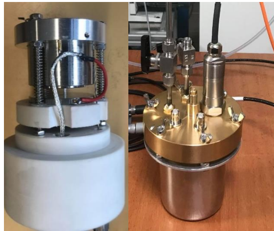
Figure 95: Photographs of the dielectric tests cell used during this study. left: interior part of oil-paper dielectric test cell. Right: complete oil-air dielectric test cell.
