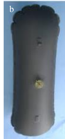
Figure 15: a: Schematic view of liquid preservation systems in Power Transformers, b: rubber bladder found inside the expansion tanks. Extracted from the Electrical Power Transformer engineering handbook [3].
