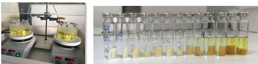
Figure 32: On the left; ageing of head space vials in oil bath (the first batch was protected from light by adding boxes on top of the stirrers; for the other experiments vials were wrapped in aluminum foil). On the right; vials of BKP samples aged from 3 hours to 13 days at 130 °C.
