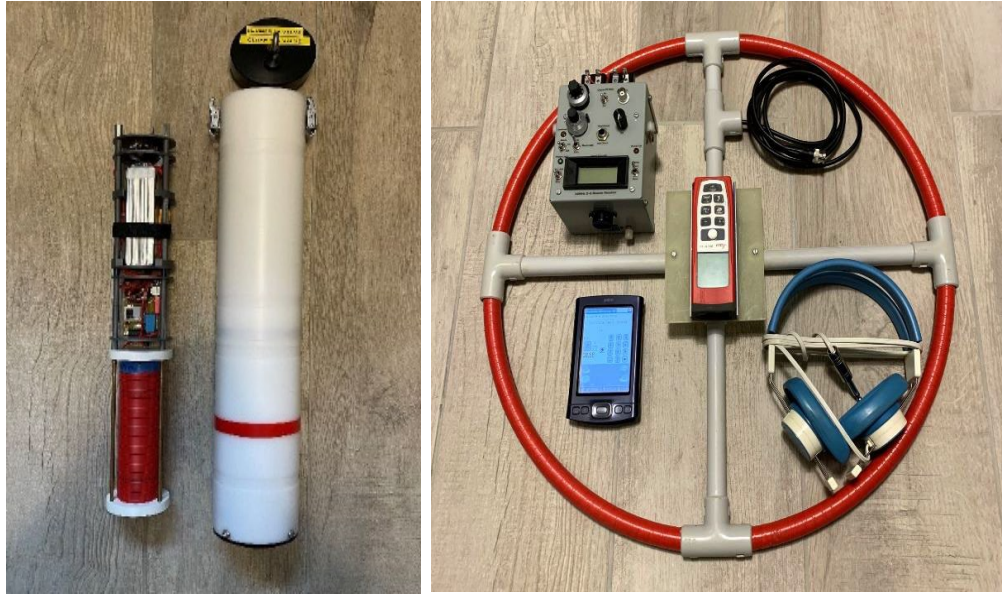
Figure 3. 6 The transmission beacon transmits at 3496 Hz. The coil (red solenoid) produces the magnetic field generated by the oscillator (center). The power supply is a 4-cell 5Ah Ph. D.C. LiPo battery. The receiving equipment, including the receiver, the antenna, the high impedance headphones, the Palm which runs the Radioloc 3D application, and the DistoX for measuring the field angle Ph. D.C from Daniel Chailloux.
