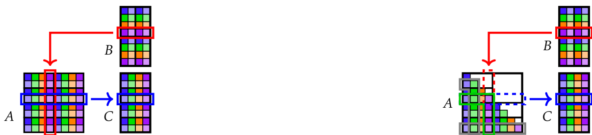
Figure 2.10 – Communications incurred with an A -stationary matrix multiplication, with a 2D BC (2, 4) distribution. Left: storing the whole matrix A . One block of B follows the red path and is sent to p - 1 = 1 nodes. A result computed on a row of A is involved in a reduction operation on q nodes (blue path), resulting in q - 1 = 3 messages sent. Right: storing the lower half of A . Both types of communication now involve p + q - 1 = 5 nodes, resulting in 4 messages sent. Parts of the matrix where fewer nodes are involved are highlighted in grey.
