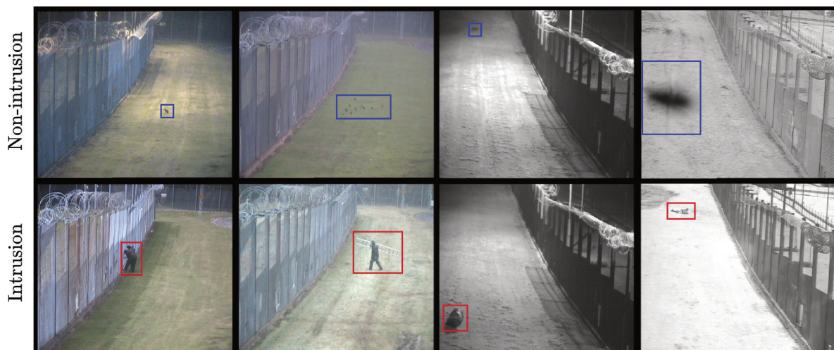
Figure 1.8: Example frames drawn from i-LIDS sterile zone dataset with various intrusion (intruders in red boxes) and non-intrusion frames. The color and black and white frames belong to view 1 and view 2 respectively. The time of the day in four columns are dawn, dusk, night, and day. The distractions (in blue boxes) in non-intrusion row (left to right order) are a rabbit, birds with rain, fox and an insect on camera respectively. In intrusion row (left to right order), we have two intruders, intruder with ladder during snow, log rolling intruder and crawling intruder respectively.
