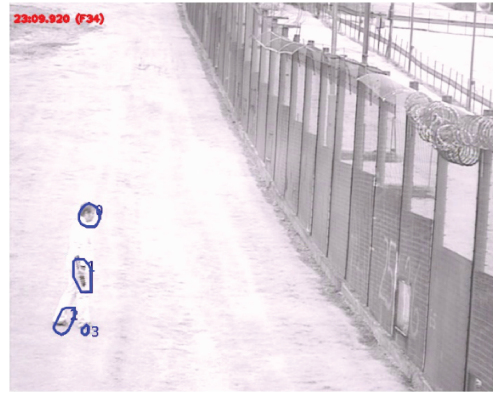
(b) Object split into extra detections in i-LIDS dataset. Blue blobs show split-object detections along with their index number.
