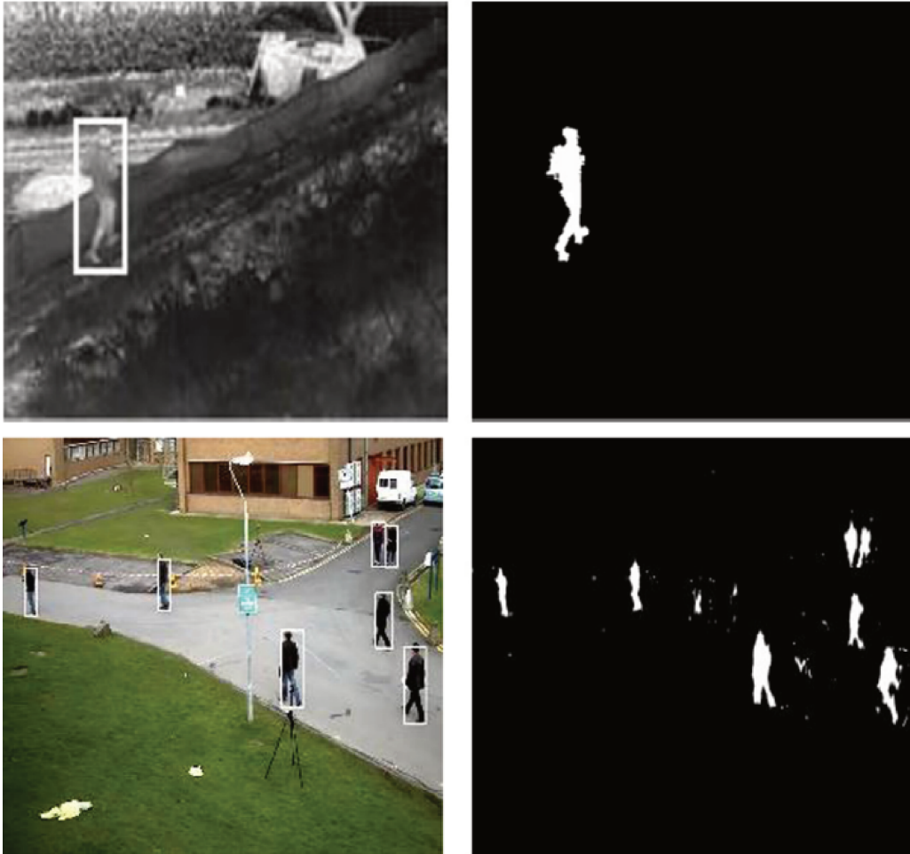
Figure 2.23: Moving object detection using background subtraction proposed by Kim et al. (2018b). The first column represents frames from a thermal and color camera respectively, with objects of interest in white bounding boxes. The second column demonstrates the output after background subtraction and image binarization, where white regions represent detected moving objects.
