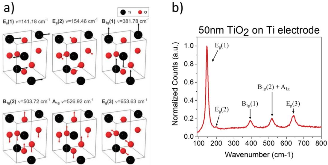
Figure II. 19: Raman spectroscopy experiment on anatase-phase TiO<sub>2</sub>. a) Scheme of Raman active atomic vibrations in anatase TiO<sub>2</sub> (the arrows represent the amplitudes of vibrations) [24]. b) Raman spectrum of 50 nm TiO<sub>2</sub> anatase measured at 25 °C.
