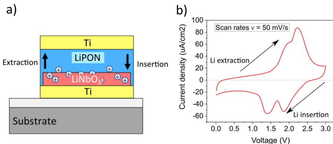
Figure V. 8: Preliminary study of  $\text{LiNbO}_3$  as an active channel material. a) The battery-like test structure composed of  $\text{Ti}/\text{LiNbO}_3/\text{LiPON}/\text{Ti}$ . b) The voltammogram of the test device confirms the functionality of the gate stack.
