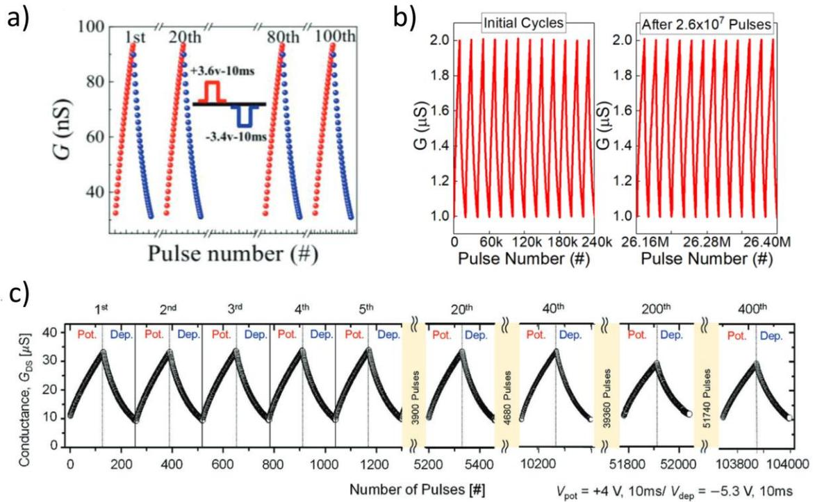
Figure I. 12: Endurance test of SynTs. a) 100 cycles of channel conductance switching with 32 discrete states induced by asymmetric  $V_G$  pulses [44]. b) Demonstration of endurance for 1300 cycles and  $2.6 \times 10^7$  pulses on a SynT using a conditioned cycling measurement, and the device still works after the last cycle of this test [51]. c) A SynT demonstrated with  $> 10^5$  writing operations and the evolution of the highest conductance value  $G_{max}$  over the cycles [44].
