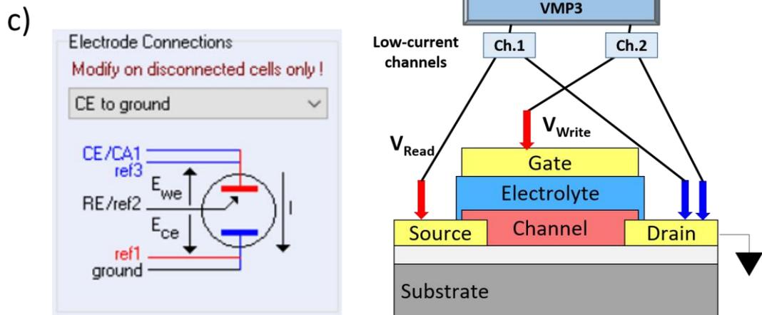
Figure III. 7: a) The electrical setup used to characterize electrochemical systems in this thesis. Schematic illustration of b) a two-terminal structure measurement and c) a transistor measurement.
