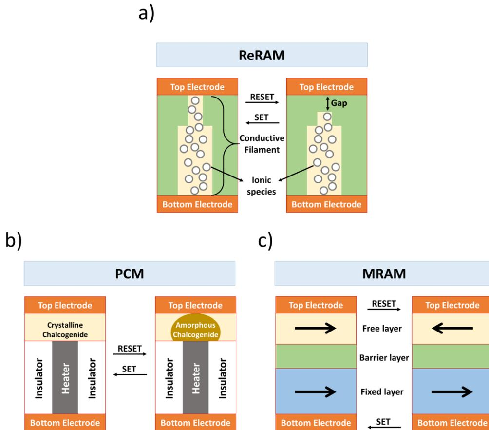
Figure I. 4: Memristor devices. a) Resistive random access memory (ReRAM). b) Phase change memory (PCM). c) Magnetoresistive random access memory (MRAM).
