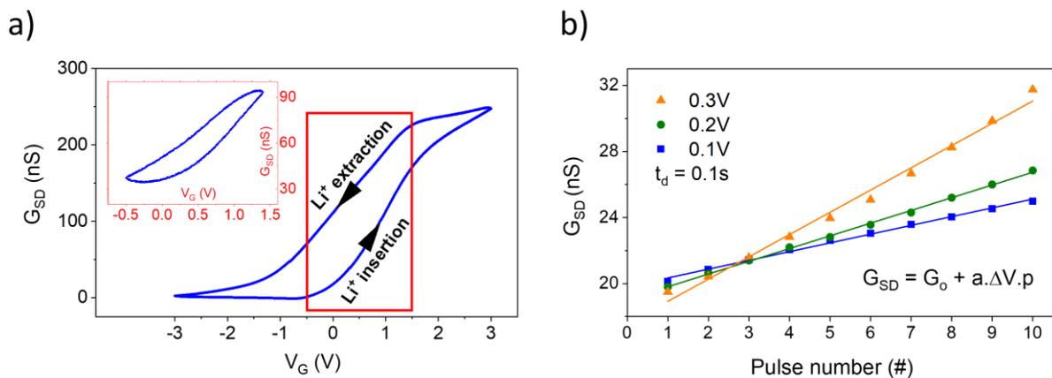
Figure III. 13: a) Charge transfer curve (channel conductance  $G_{\text{SD}}$  as a function of gate voltage  $V_{\text{G}}$ ) with a gate sweep of 50 mV/s in the potential range [-3 V, 3 V] (inset: Focused working window of [-0.5 V, 1.5 V]). b) Conductance  $G_{\text{SD}}$  change under incremental voltage amplitude pulses from 100 mV to 300 mV with a duration  $t_d$  of 0.1 s.
