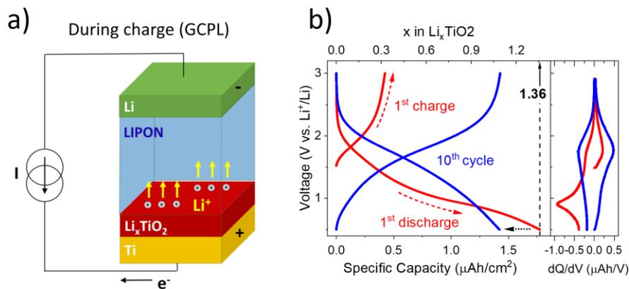
Figure III. 19: a) Schematic view of  $\text{Ti}/\text{Li}_x\text{TiO}_2/\text{LiPON}/\text{Li}$  vertical structure during GCPL charge process. b) Comparison of 1<sup>st</sup> and 10<sup>th</sup> cycle upon GCPL (The cell is charged to 3.0 V and discharged to 0.5 V with the current density of  $\pm 2.6 \mu\text{A}/\text{cm}^2$ ).
