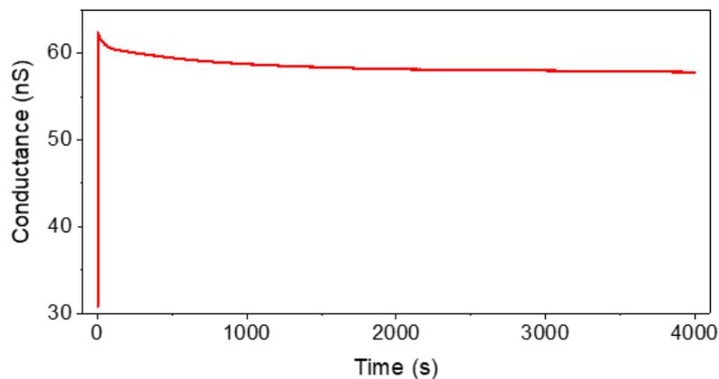
Figure III. 15: Retention profile of a conductance state over 4000 s.
