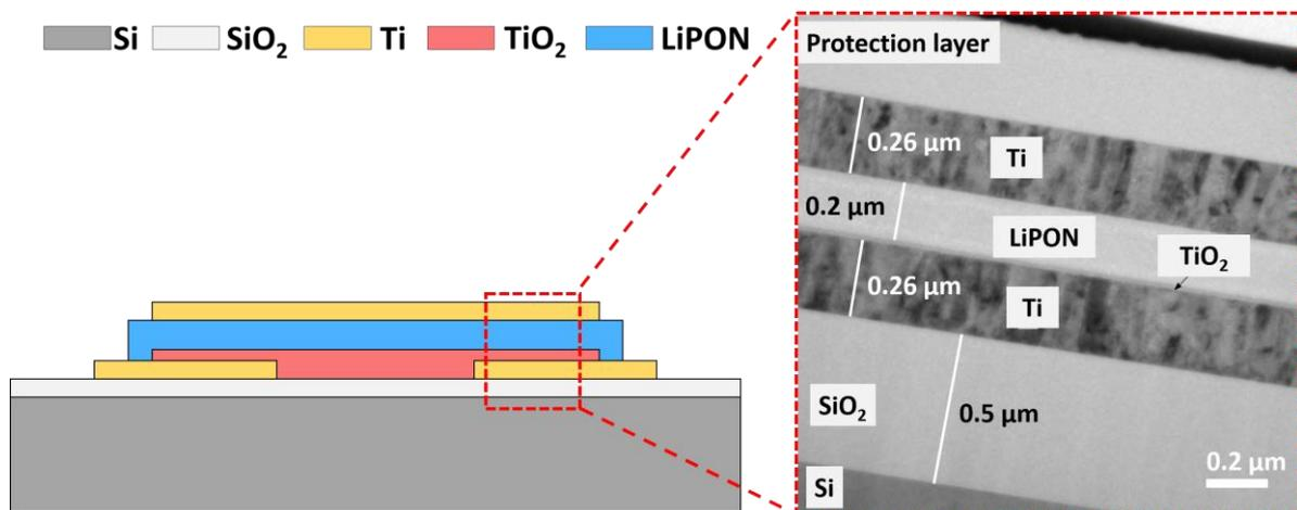
Figure II. 24: Cross-section TEM image of a SynT made of Ti electrodes,  $\text{TiO}_2$  channel, and LiPON electrolyte.
