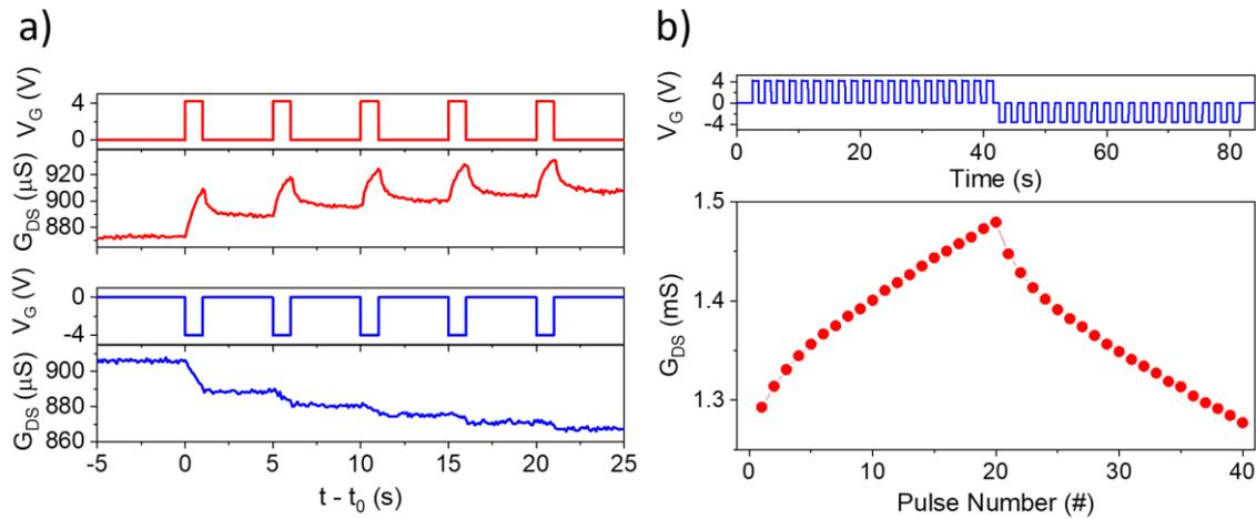
Figure III. 10: a) Analog conductance modulation demonstrated with five pulses of  $V_G = +4.2$  and  $-4.0$  V amplitude and 1 s duration. b) One cycle of conductance modulation with 40 pulses of potentiation and depression pulses.
