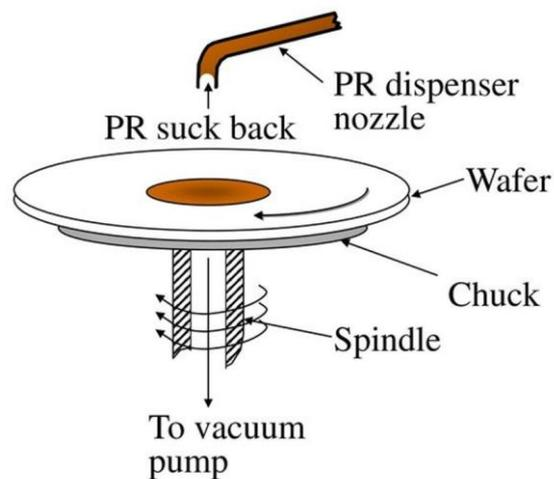
Figure II. 9: Schematic of a photoresist automatic dispenser [13].
