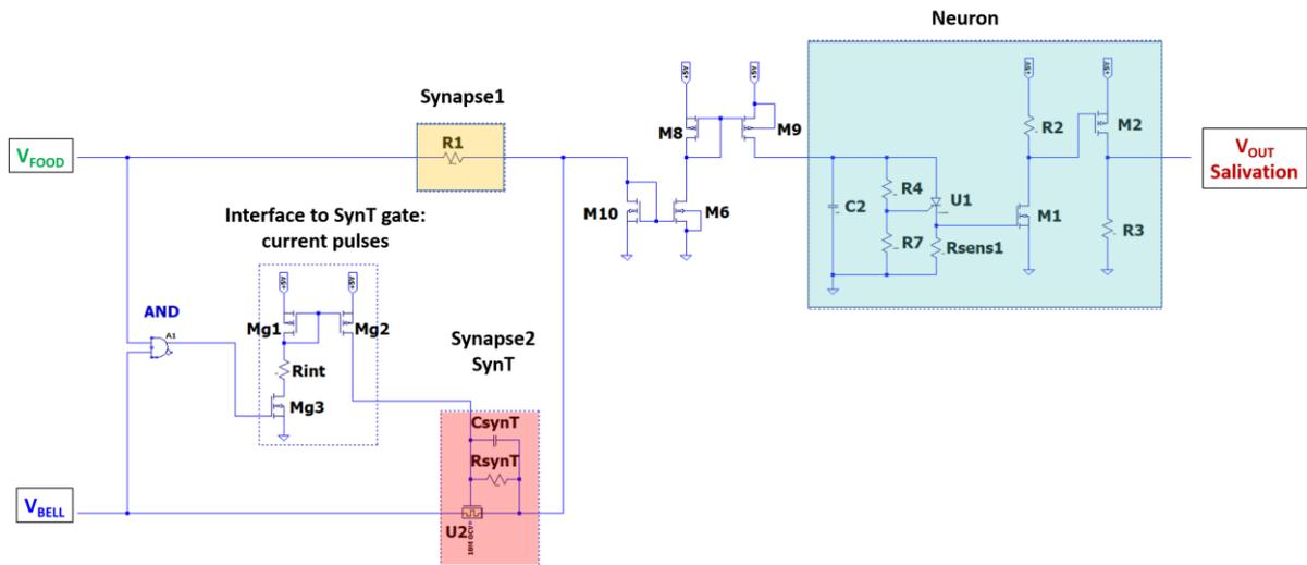
Figure IV. 18: Schematic of the whole circuit: when  $V_{FOOD}$  and  $V_{BELL}$  arrive simultaneously to the AND component, the latter delivers a 5V voltage output, which is converted to a (in the nA range) current arriving at the gate of synapse2 (SynT): this results in a gradual increase of the SynT conductance.
