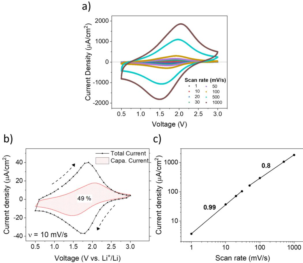
Figure III. 22: a) Cyclic voltammetry of  $\text{TiO}_2/\text{LiPON}/\text{Li}$  half-cell at increasing scan rates from 1 to 1000 mV/s. b) CV study at 10 mV/s and the calculated pseudocapacitive current contribution. c) Logarithmic relationship between cathodic peak current ( $\text{Li}^+$  insertion) and scan rates between 1 mV/s and 1 V/s.
