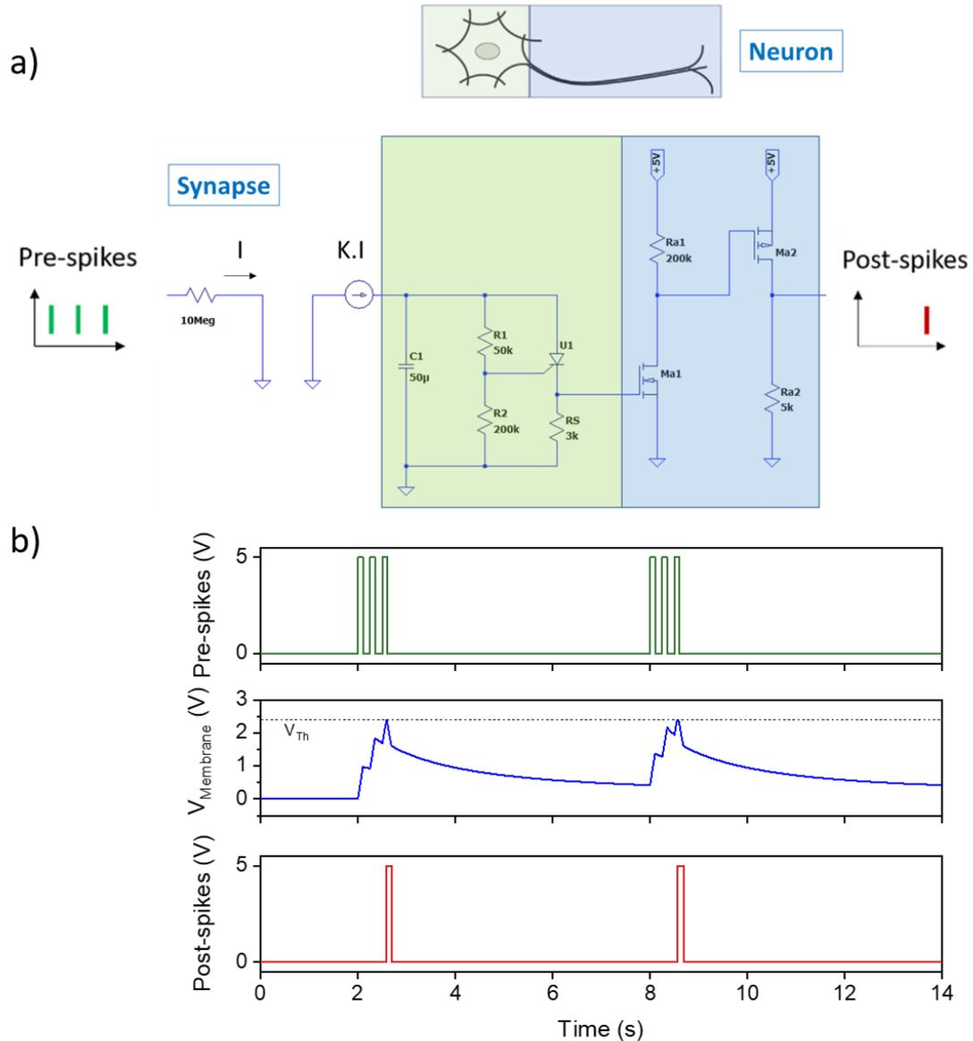
Figure IV. 16: a) Illustration of Leaky integrate-and-fire neuron model circuit and b) its electrical response to pre-spikes.
