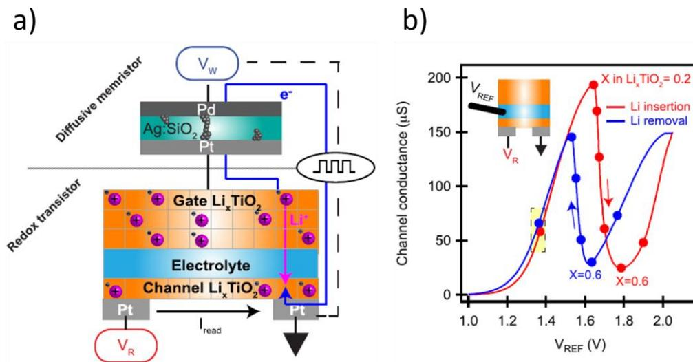
Figure III. 5: a) An electrochemical synaptic transistor made of an anatase-phase  $\text{Li}_x\text{TiO}_2$  channel. b) The conductance variation of the channel under the change of Li content. Adapted from [4].
