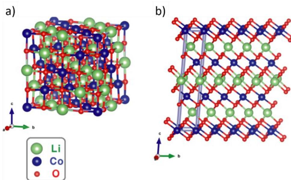
Figure III. 1: Crystal structures of (a)  $Fd\bar{3}m$  spinel  $\text{LiCoO}_2$  (LT-LCO) and (b)  $R\bar{3}m$  layered  $\text{LiCoO}_2$  (HT-LCO) [17].
