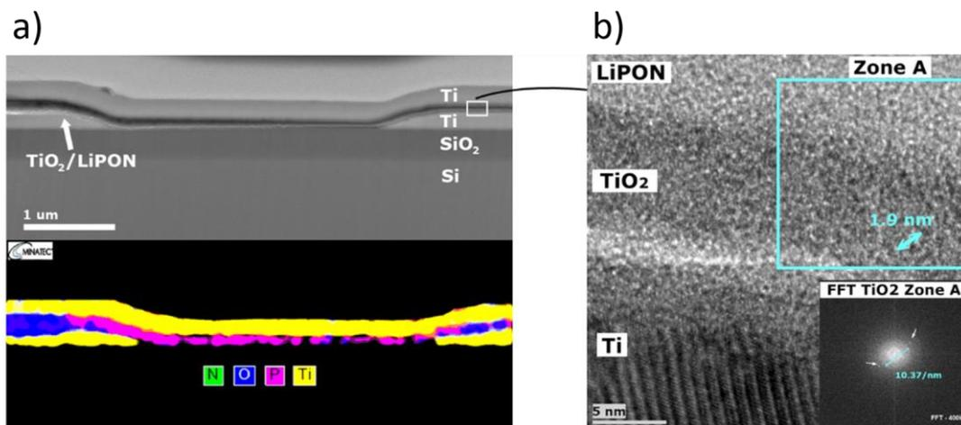
Figure III. 12: a) SEM and EDS characterizations of SynT's gate stack. b) HRTEM image with the focus on the neighborhood of TiO<sub>2</sub> channel (inset: FFT on the selected Zone A)
