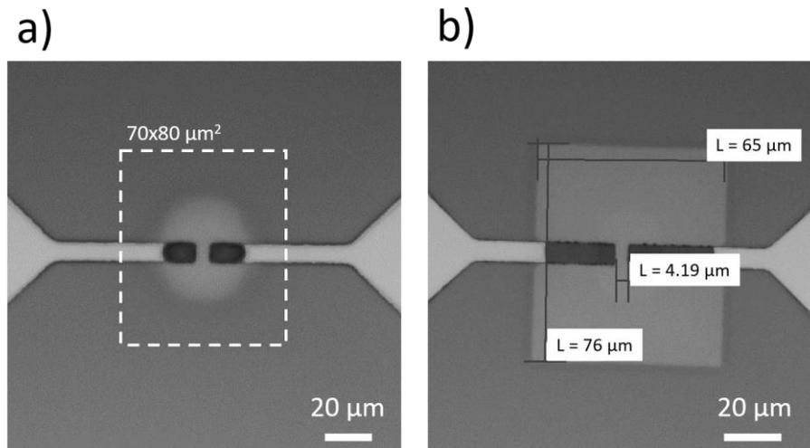
Figure II. 28: a) Lateral over-etching of LCO thin film with the dashed square being the patterned photoresist mask. b) An improved patterning of LCO channel with 5  $\mu\text{m}$  over-etched on each side.
