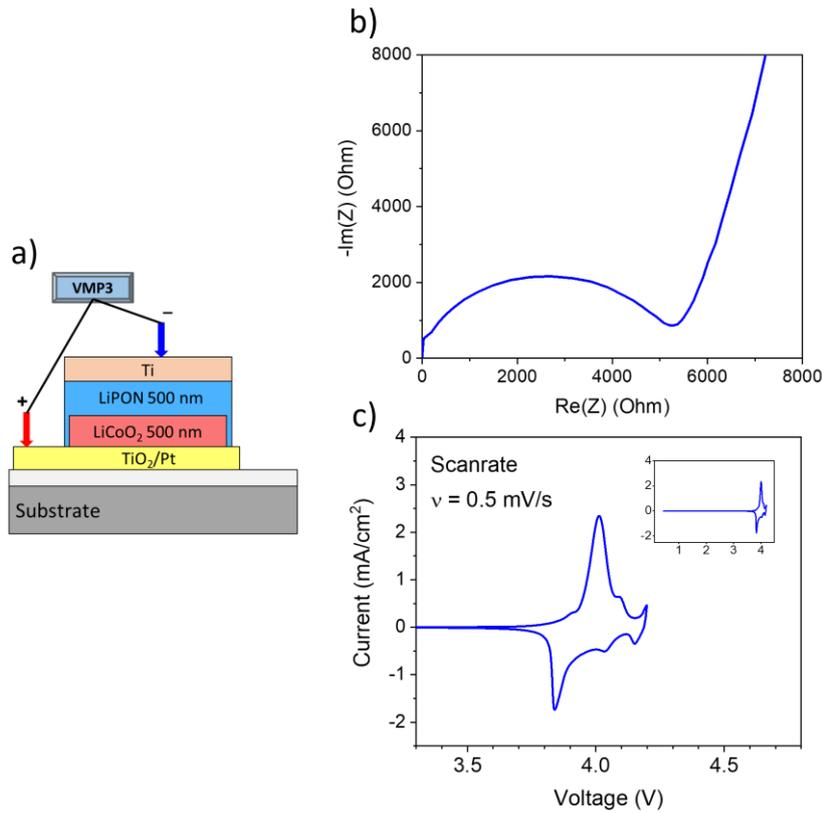
Figure III. 8: Electrochemical study of LiCoO<sub>2</sub>/LiPON gate stack. a) The illustration of the battery-like structure used. b) EIS study of a test structure with an area of 1.13 mm<sup>2</sup>. b) CV study of the same device showing the redox potentials.
