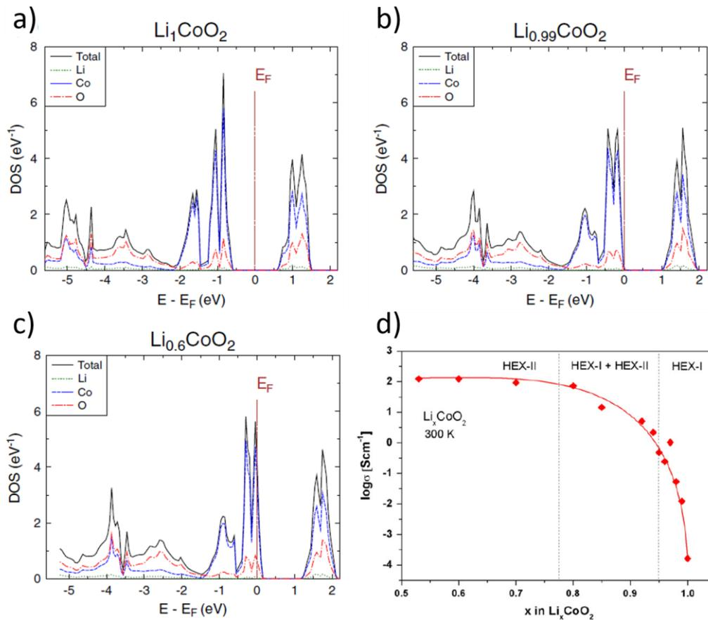
Figure III. 2: Total and site-decomposed DOS of  $\text{Li}_x\text{CoO}_2$  oxides with different Li concentration, i.e. a)  $x=1$ , b)  $x=0.99$ , and c)  $x=0.6$ . d) Variation of the electrical conductivity of  $\text{Li}_x\text{CoO}_2$  at 300 K as a function of lithium concentration  $x$ . Adapted from [19].
