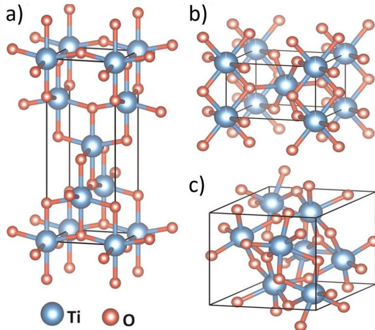
Figure III. 3: Crystal structures of  $\text{TiO}_2$  (a) anatase (tetragonal), (b) rutile (tetragonal), and (c) brookite (orthorhombic) polymorphs [26].
