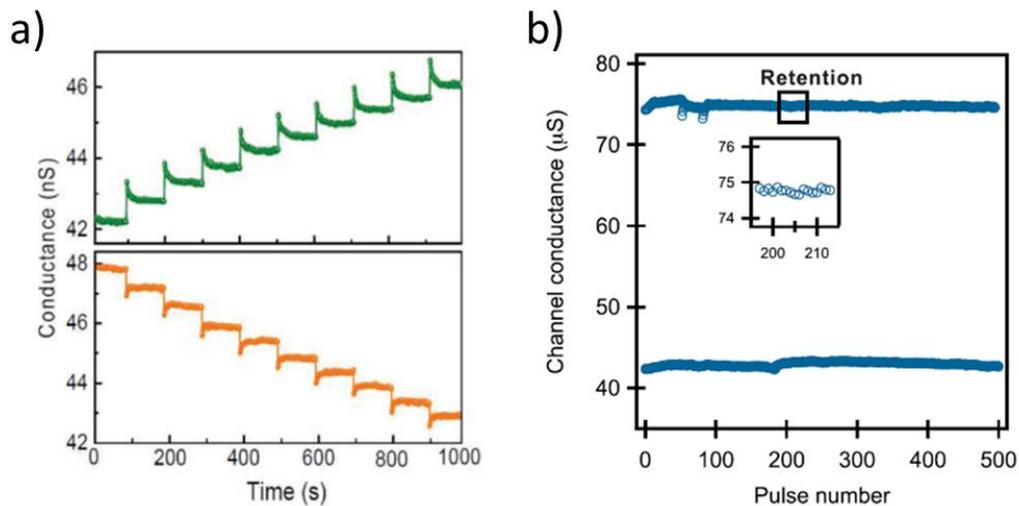
Figure I. 10: Analog state retention of synaptic transistors. a) Retention of the  $\alpha$ - $\text{MoO}_3$ -based channel conductance states for LTP (top) and LTD (bottom) in periods of 100 seconds [31]. b) The retention of more than 500 seconds of single states (highest and lowest) measured on a 1S1T device after the selector is switched off (each pulse represents 1 s) [49].
