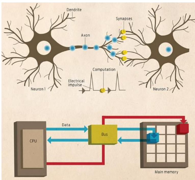
*Figure 1. 1: Brain versus Computer. (Top) Neurons in human brain are connected via billions of neural connections – synapses, creating a biological computer with energy- and time-efficient computing ability. (Bottom) Conventional computer structure with memory and processing units separated. This structure requires data to be shuttled between the two units and thus, the data latency is unavoidable [2].*
