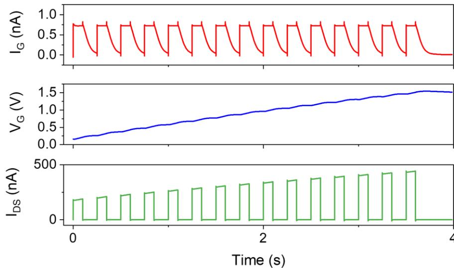
Figure IV. 21: Simulation of the SynT response (Top) The writing current pulses. (Middle) The increase of gate potential (simulated by the potential across  $C_{SynT}$ ). (Bottom) The channel current  $I_{DS}$  of SynT.
