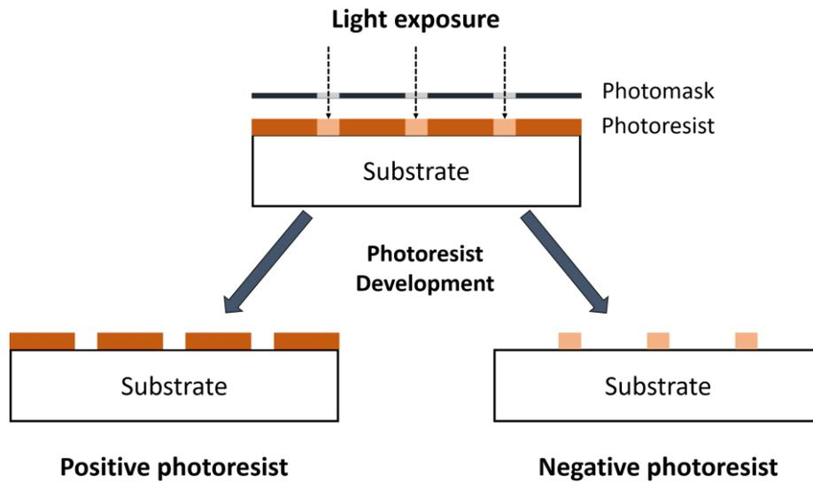
Figure II. 10: Two types of photoresist: positive and negative.
