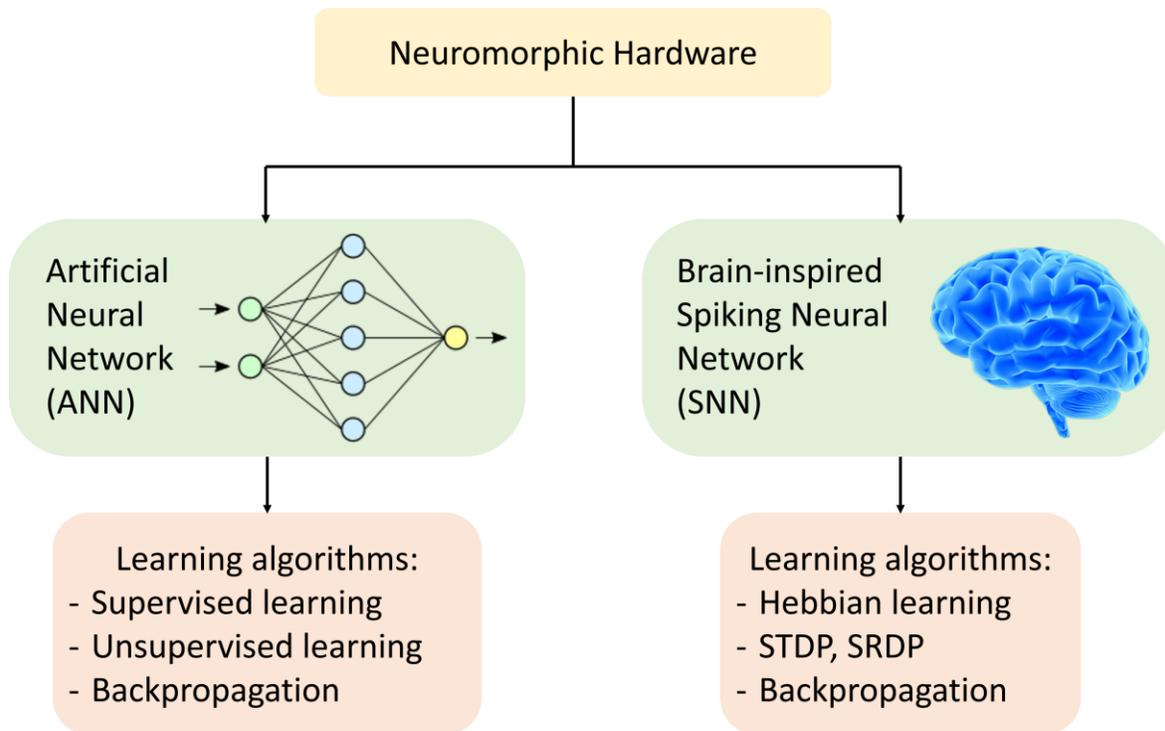
*Figure 1. 3: Neuromorphic hardware can be implemented via both artificial neural networks (ANNs) and brain-inspired neural networks. These two approaches rely on a different set of algorithms and learning rules, e.g. the backpropagation algorithm in ANNs, or the temporal dynamics in brain-inspired SNN concepts.*
