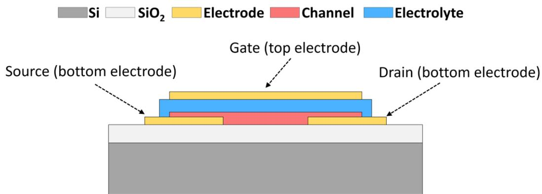
Figure II. 1: Schematic view of the synaptic transistors elaborated.
