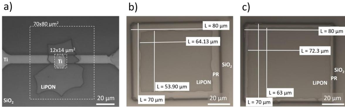
Figure II. 30: a) Result of gate electrode and electrolyte patterning at the beginning of the thesis. Wet etching of 100 nm LiPON layer on SiO<sub>2</sub> during b) 45 s + 5 s rinsing with DI water, and c) 32 s + 5 s rinsing with DI water.
