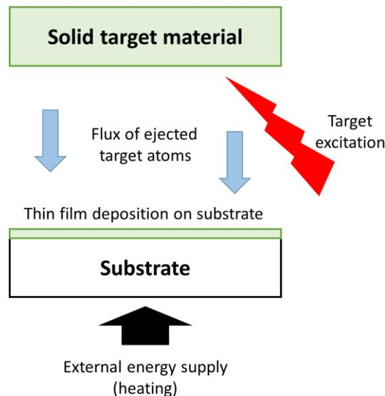
Figure II. 3: Physical vapor deposition working principle. Adapted from [2].
