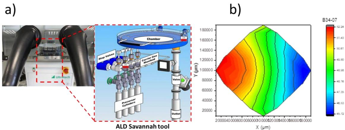
Figure II. 7: a) ALD deposition tool and the schematic of the parts. Adapted from [12]. b) A thickness mapping by ellipsometry on  $50\text{ nm TiO}_2$  film grown on  $\text{SiO}_2$ .
