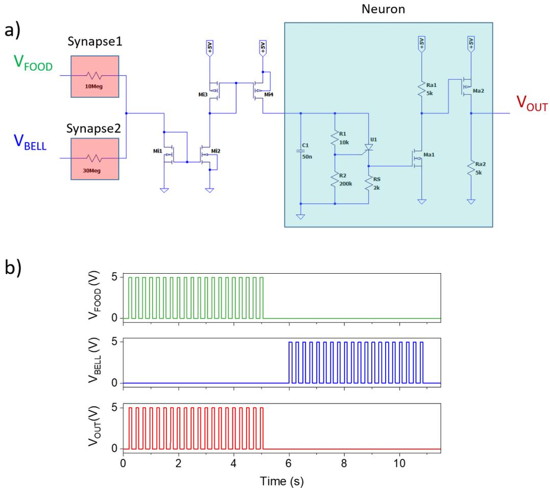
Figure IV. 17: a) Circuit with two synapses (resistors of 10 M $\Omega$  and 30 M $\Omega$ ) in red, and the LIF neuron circuit in green b) Simulation results of the evolution of the V<sub>OUT</sub> voltage, as a function of V<sub>FOOD</sub> and V<sub>BELL</sub>.
