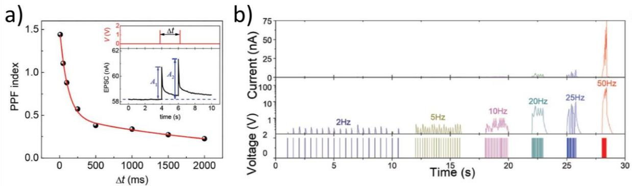
Figure I. 13: Temporal dynamics demonstrated on SynTs. a) Paired-pulse facilitation (PPF) ratio measurement on an  $\alpha$ - $\text{MoO}_3$ -based SynT represents STDP characteristics [31]. b) The current (weight) change in linear scale (top panel), log scale (middle panel) in  $\text{WSe}_2$  based synaptic transistors as a function of the frequency of gate pulses, implying SRDP behavior [47].
