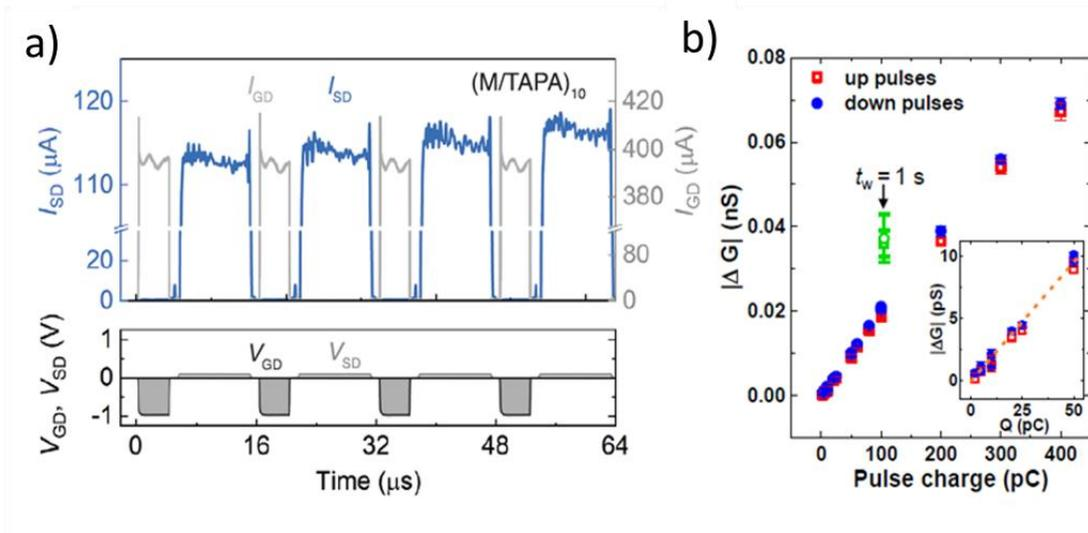
Figure I. 11: Current measurements for energy calculation. a) The pulses scheme for GS and DS electrodes (bottom), and the resulted current measurement. The  $I_{SD}$  represents the analog states and  $I_{GD}$  represents the flow of charge transferred [57].
