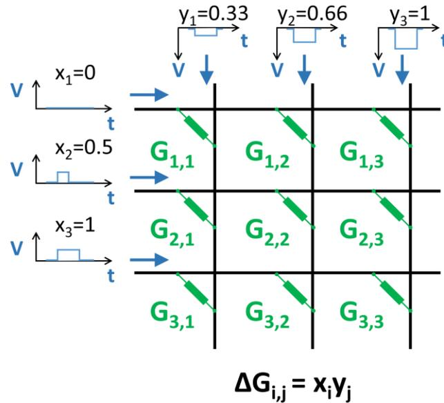
Figure IV. 7: Illustration of parallel weight update during training.
