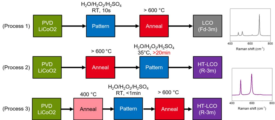
Figure II. 29: Evolution of processes to obtain HT-LCO channel layers.
