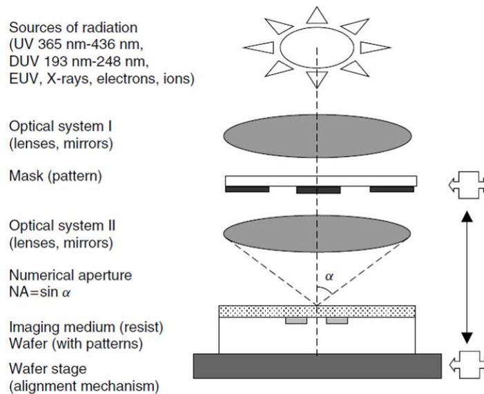
Figure II. 8: Schematic of an optical lithography aligner/exposure tool [2].
