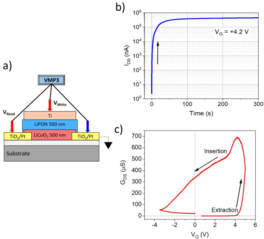
Figure III. 9: Electrical test of the synaptic transistor. a) The illustration of the SynT with a 500-nm LiCoO<sub>2</sub> channel and 500-nm LiPON electrolyte. b) The evolution of channel conductance under a constant extraction of Li ion at  $V_G = 4.2$  V. c) Hysteresis conductance profile of the channel under Li intercalation.
