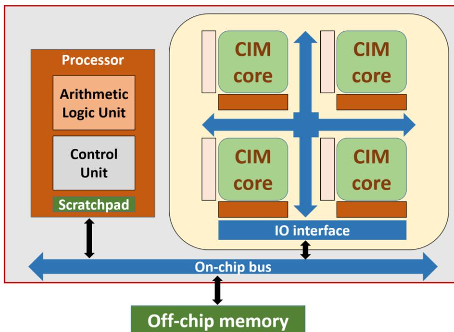
Figure IV. 5: Computing in memory structure [21].
