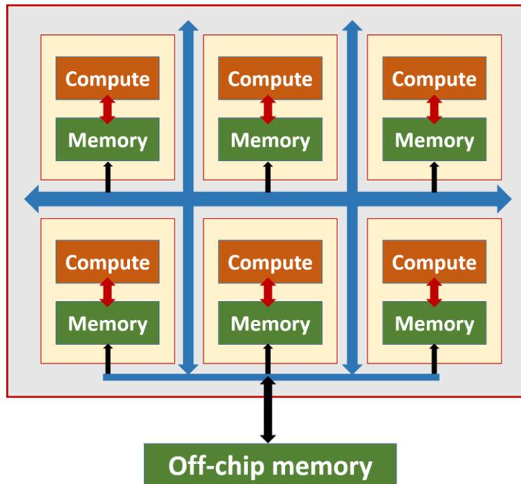
Figure IV. 4: Computing near memory structure [21].
