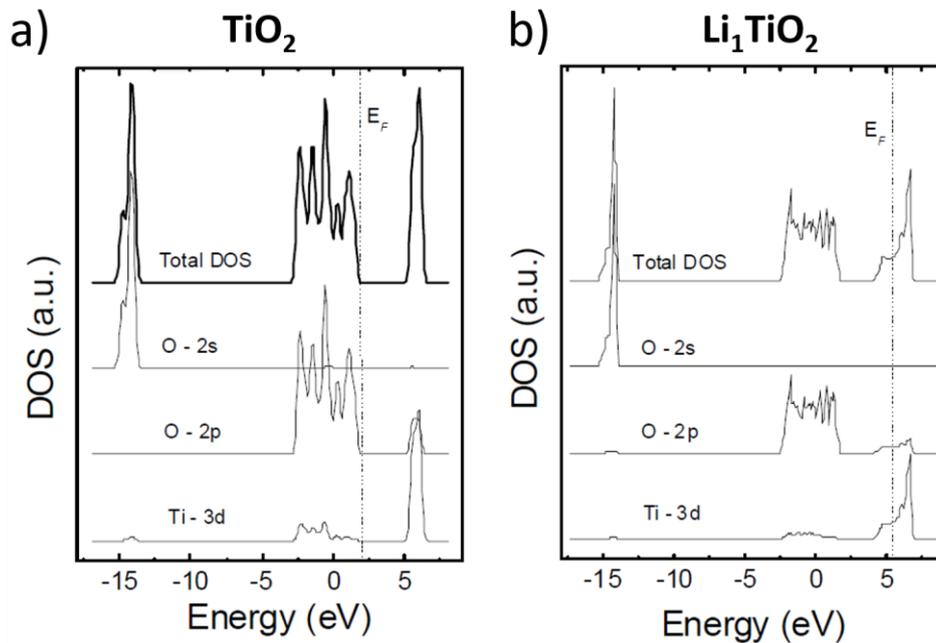
Figure III. 4: Total density of state of anatase-phase a)  $\text{TiO}_2$  and b)  $\text{Li}_1\text{TiO}_2$  anatase respectively related to the partial DOS of atomic orbitals of Ti and O.
