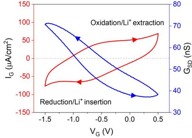
Figure III. 21: SynT channel conductance modulation (blue curve) and gate current response (red curve) as functions of the sweeping of gate voltage.
