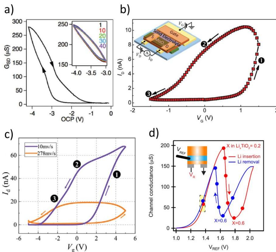
Figure I. 7: Conductance modulation of channel layer under Gate voltage sweeps. a)  $\text{Li}_x\text{CoO}_2$  channel SynT works in the range of under 300  $\mu\text{S}$  [30]. b)  $\alpha\text{-MoO}_3$  channel SynT works in the range of under 240 nS [31]. c)  $\alpha\text{-Nb}_2\text{O}_5$  channel SynT works in the range under 700 nS or 200 nS depending on the sweep rate [44]. d) Anatase  $\text{Li}_x\text{TiO}_2$  channel SynT works in the range of under 200  $\mu\text{S}$  [49].
