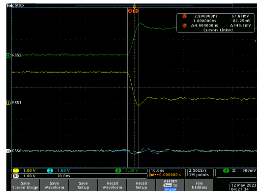
(b) Simultaneously activating the arbiter inputs IN1 and IN2 (circuit 7.3), yields Cell2 as the winning cell in no longer than 4.6ns
