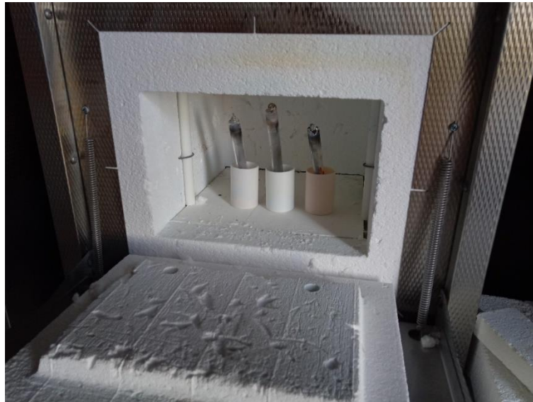
Figure III-9: Muffle furnace I used at CRISMAT with 3 samples loaded inside with alumina crucibles.
