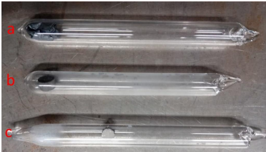
Figure III-11: Picture of quartz tubes with reacted sample after a furnace sintering. On the top the sample was rounded in a Ta foil while the 2 others were not. The consequence is the loss of Selenium deposited on the quartz tube (white smoke)
