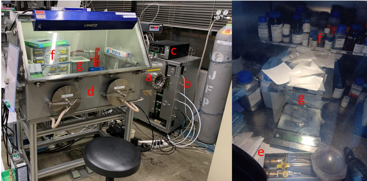
Figure III-6: A picture of the tool box I used at AIST (left) and at CRISMAT (right). We can see the different important materials used for the preparation of samples: the vacuum airlock to enter the materials (a), the pipe/pump system to control the GB's atmosphere (b), the oxygen level controller (c), the access holes with gloves (d), the working space with the tools (e), the powders racks (f), the weight machine (g) and the hydraulic press (h).
