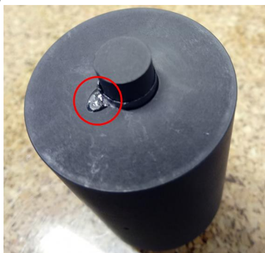
Figure III-25: Picture of the carbon mold used to prepare SPS sample at CRISMAT. We can see, in the red circle, a Selenium droplet which was ejected during the in-situ process using the 1:1.5 stoichiometry.
