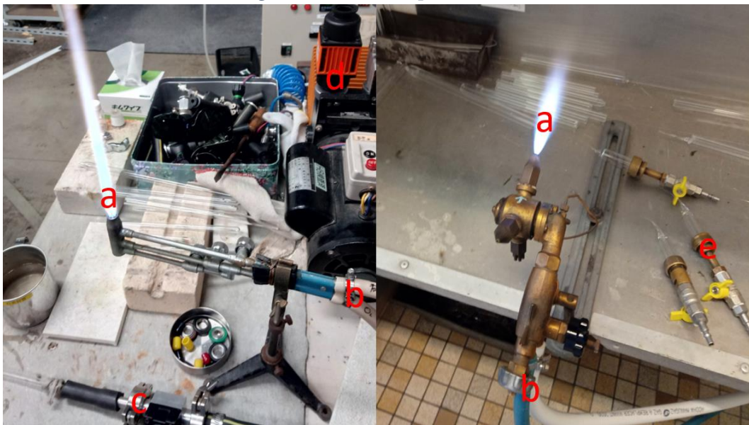
Figure III-8: Pictures of the torch and the pipe/pump system to melt and seal the quartz tube used at AIST (left) and at Caen (right). We can see the flames at roughly 1300 °C (a), the pipe bringing the gas and the oxygen for the combustion (b), a quartz tube with the sample plug on the pump before the sealing (c), the pump (d) and the remaining quartz tube after the sealing (e).
