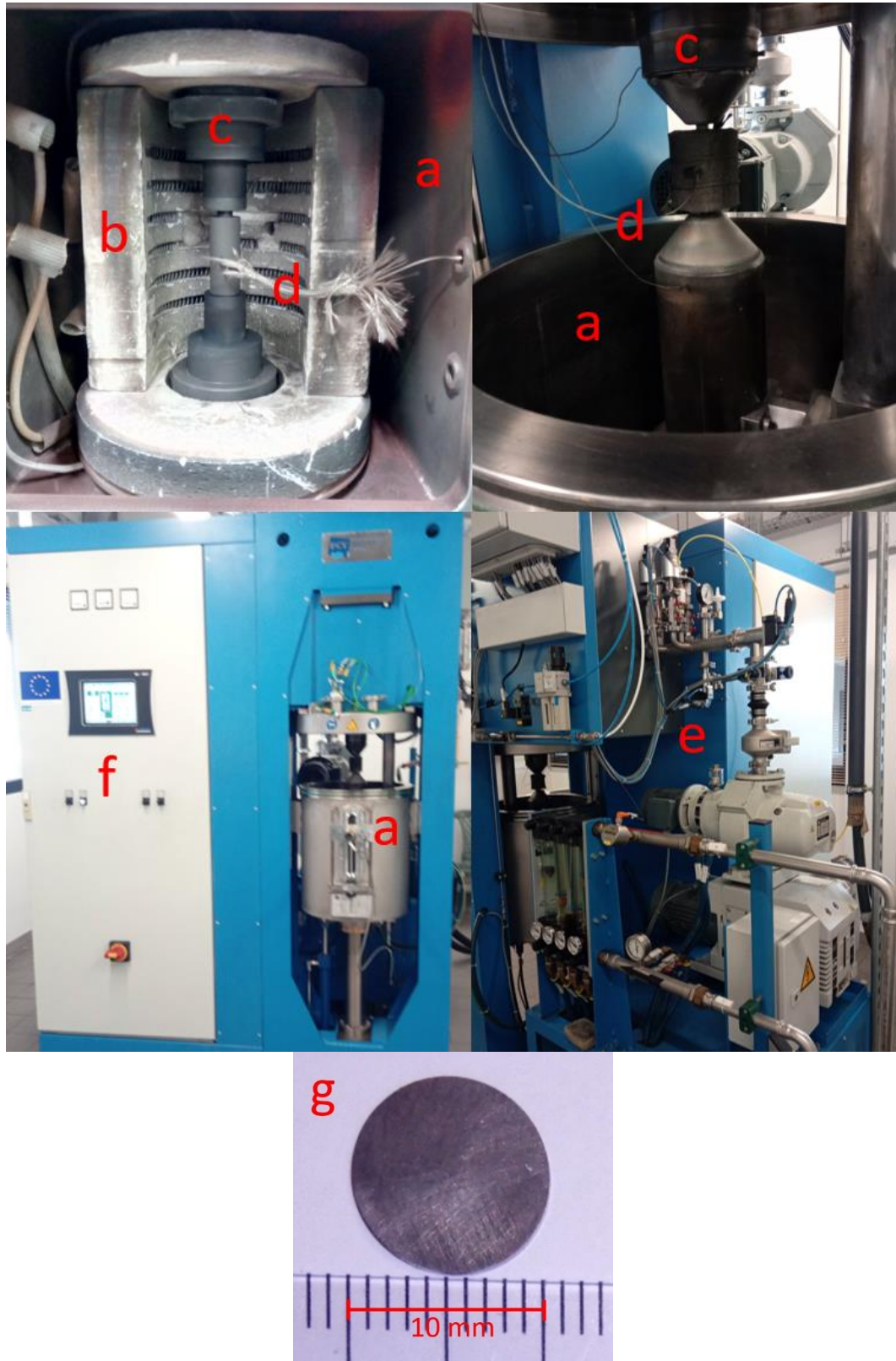
Figure III-13: Pictures of the vacuum chamber (a) of the SPS machines used at AIST (top left) and CRISMAT (top right). The AIST machine possesses a Hot-Wall (b) which allows a Hot-pressing process. We can see the current leads (c) and the thermocouple used to measure the temperature (d). The 2 others pictures are the face and the back of the SPS machine used at CRISMAT with the pump/pipe system (e) and the control panel (f). A 10 mm size sample after the SPS synthesis is presented at the bottom (g).
