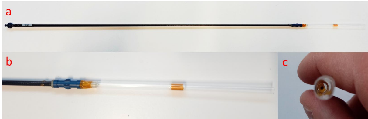
Figure II-19: (a) Sample holder of the SQUID where a straw, containing the sample, is fixed. (b) A zoom on the straw with the sample inside a cap rounded with Kapton. the straw is perforated to evacuate the air during the purge of the vent. (c) A view on the top of the straw where we can see the sample (A piece of commercial YBaCuO). The sample is laying on a Teflon leaf and trap inside a cap rounded by Kapton.
