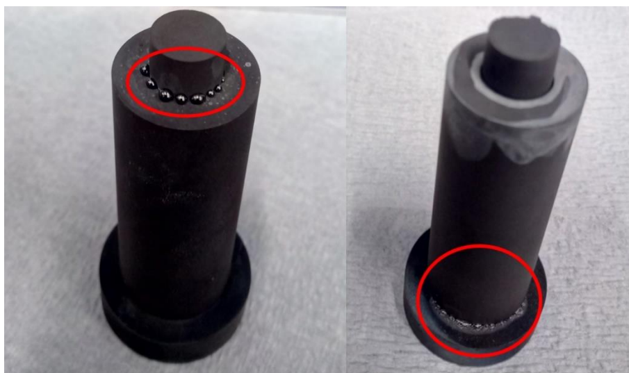
Figure III-22: Carbon molds right after the SPS sintering with an in-situ process. Selenium drops are visible outside the mold since they escaped during the synthesis process.
