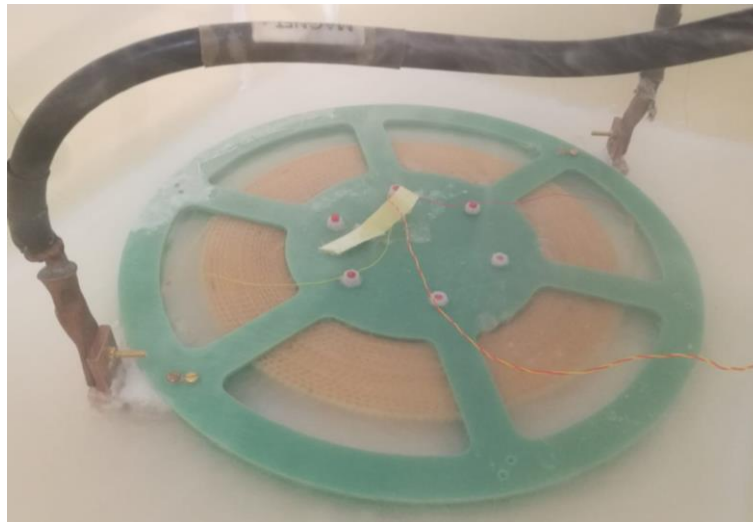
Figure I-15: Picture of a non-inductive superconducting coil made of HTS YBCO tapes for a power filter [67].
