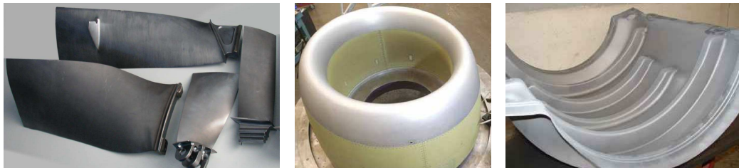
Figure 1.2 – Example of aeronautical parts manufactured with the SPF process [42]
