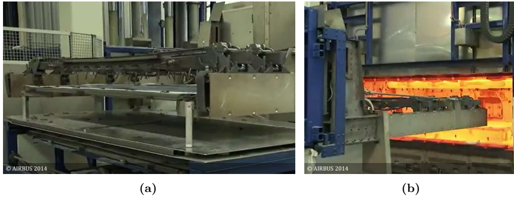
Figure 1.5 – Pictures of the press environment (a) loading step (b) unloading step
