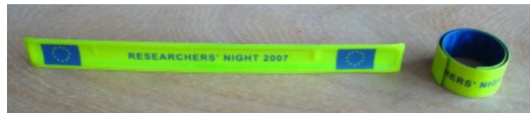
Figure 1.13: Two trouser clips, one open (left) and one closed (right), a bistable plate mechanism that uses the anisotropy
