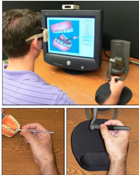
Figure 1.24: Force feedback simulator setup for dental surgery: comparison between handling the real instrument and the haptic stylus [CPT09]
