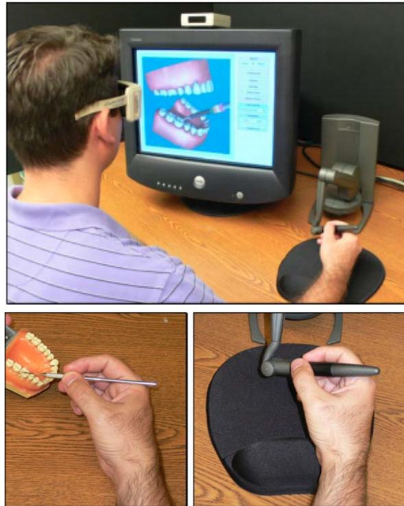
**Figure 1.24:** Force feedback simulator setup for dental surgery: comparison between handling the real instrument and the haptic stylus [CPT09]
