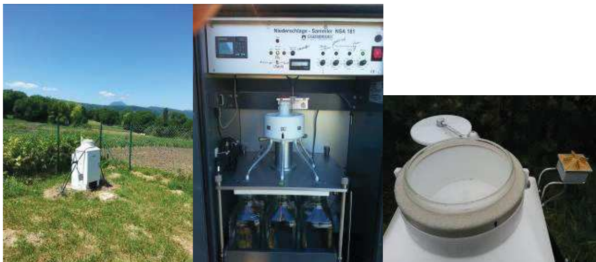
Figure 6: Wet-deposition sampler (Eigenbrodt NSA 181/KHS), Opme summer 2019.
