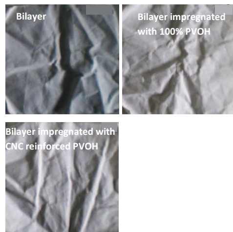
Figure 2: Crumpling pattern of pilot papers after crumpling with Balloon-test
