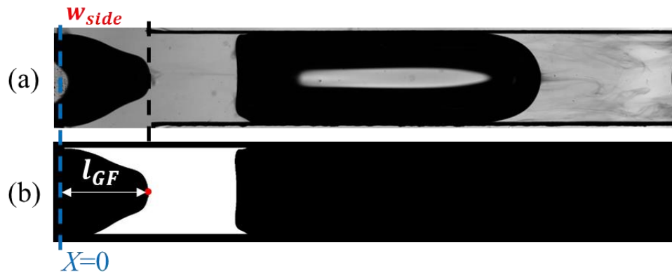
Fig. 5-5 Typical image processing for extracting gas finger right after the bubble pinch-off ( j_L = 17.9 and j_G = 25.0 \text{ cm s}^{-1} ): (a) raw image of gas finger, (b) extracted gas finger and l_{GF} represents the length of the gas finger.
