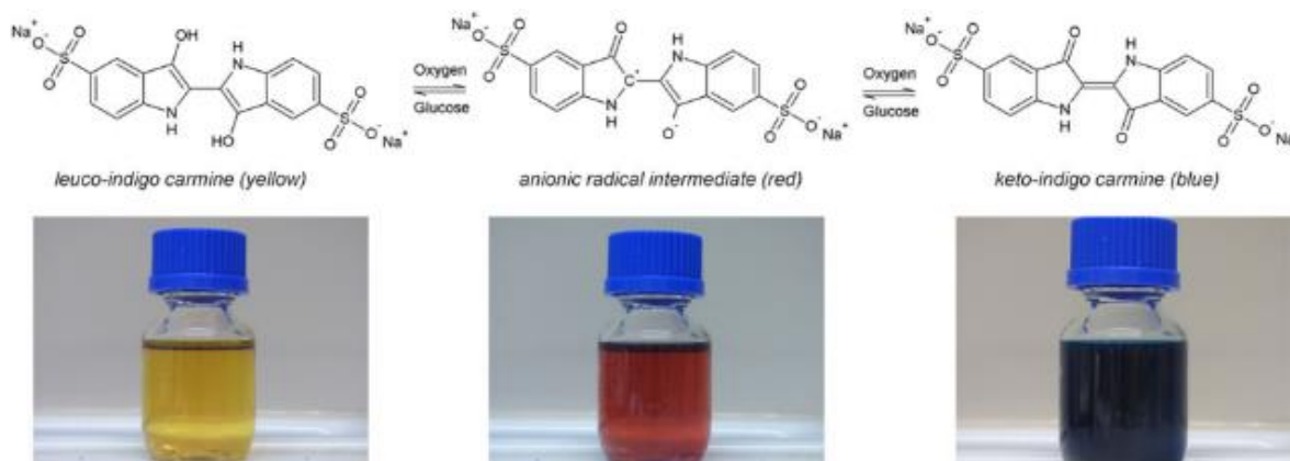
Fig. 1-18 Reversible redox reactions of leuco-indigo carmine to keto-indigo carmine with glucose as reducing agent and oxygen as oxidizing agent. Color change (yellow-red-blue) is illustrated in flask experiments. Extracted from Krieger et al. (2017).
