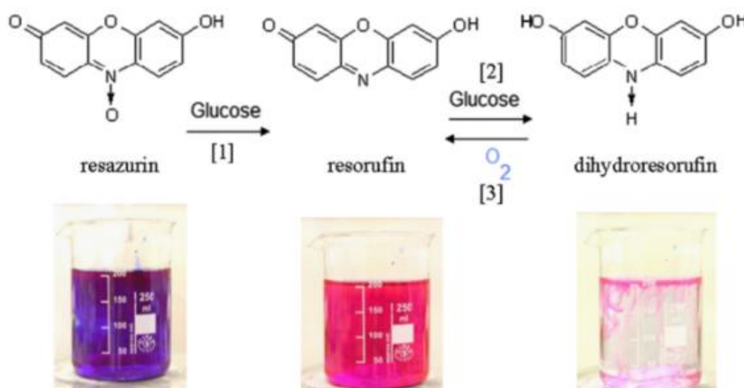
Fig. 1-17 Principles of the colorimetric method base on the use of resazurin. Extracted from Dietrich et al. (2013a)
