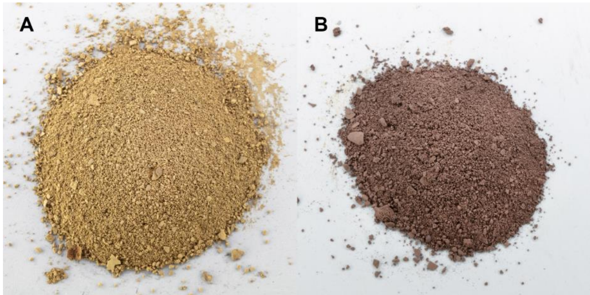
Figure 84. Photography of copper/titanium oxide mixture calcined at (A) 400°C and (B) 600°C.
