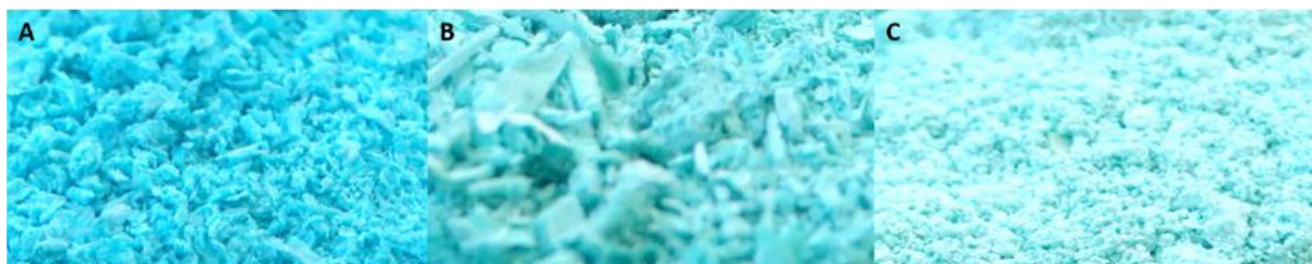
Figure 42. Macroscopic comparison of copper oxide precursor samples prepared at A) 130^\circ\text{C} ; B) 145^\circ\text{C} and C) 155^\circ\text{C} .
