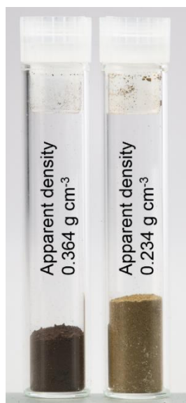
Figure 92. Comparison of the apparent densities of the pure copper oxide/titanium oxide mixtures at macroscale (CT600 left and CT400 right).
