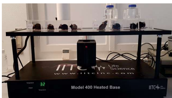
Figure 19 The plantar apparatus is composed of an emitter of a laser beam, a glass panel and animal chambers.
