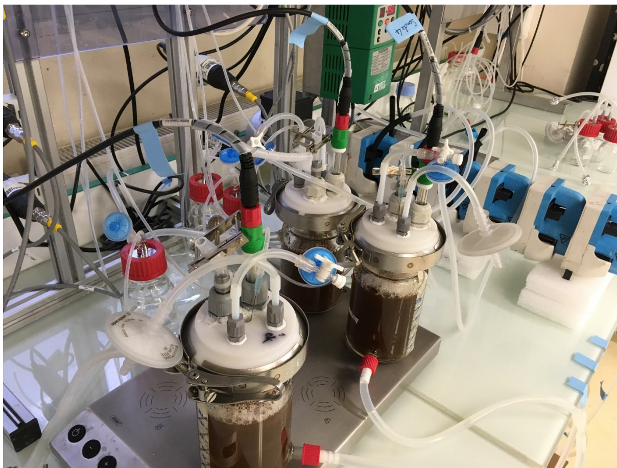
Supplementary data: Photograph of the homemade bioreactors for technical lignin degradation
