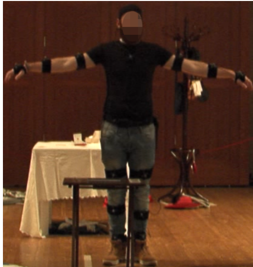
Figure 4.3: An example of “T-pose”. This pose enables the calibration of the motion capture system. Moreover, it was used as a marker for the beginning of a task and to compute the Occupied Volume feature.
