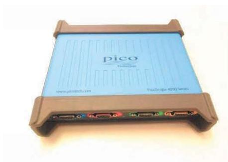
Figure 34: Picoscope 4444 oscilloscope
