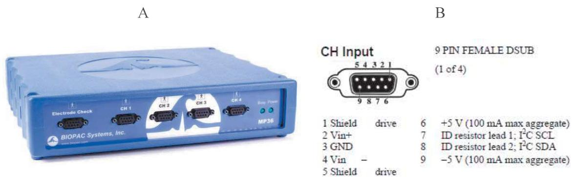
Figure 33: MP36 Biopac and its DB9 connector pinout
