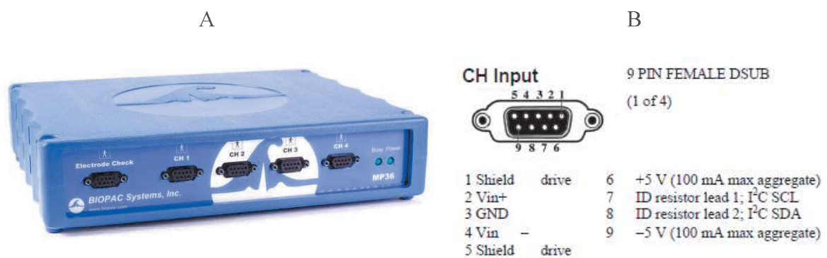
Figure 33: MP36 Biopac and its DB9 connector pinout
