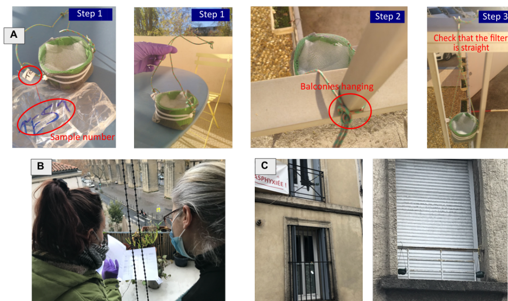
213 214 Figure 3: [a] Extract from the protocol designed to facilitate the deposimeters set up by 215 the inhabitants. [b] Protocol presentation and explanation during the kit distribution. [c] 216 Examples of the settled filters pictures sent by citizen partners.
