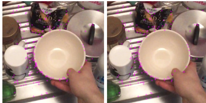
Figure 4.6: Visual comparison of detected sets of keypoints. On the left: OpenSIFT (Hess, 2010) extracted keypoints. On the right: the FPGA result.
