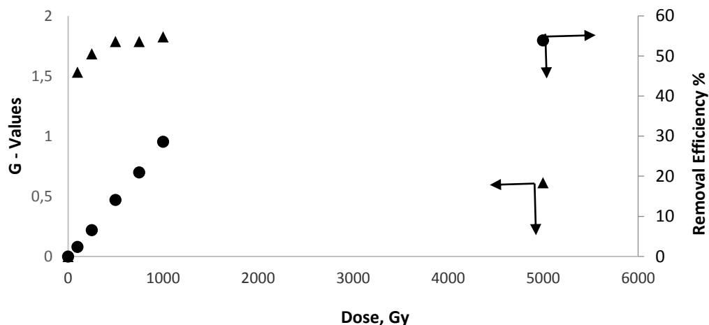
Figure 2. G-Values (▲) and removal efficiency (●) of paracetamol using gamma radiation at different doses. [Paracetamol] 0 : 100 mg L -1 , TD: 6.69 kGy h -1 , pH: 5.5.
