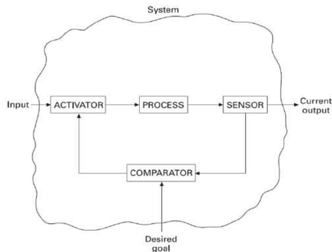
Figure 3.2. Example of a negative feedback system (Jackson, 2003)
