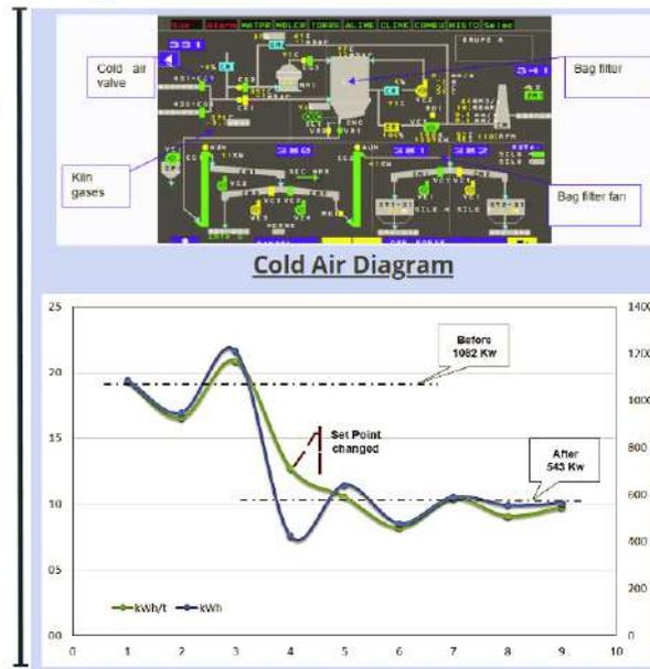
Figure 4.12. Cold Air Diagram during burning operation
