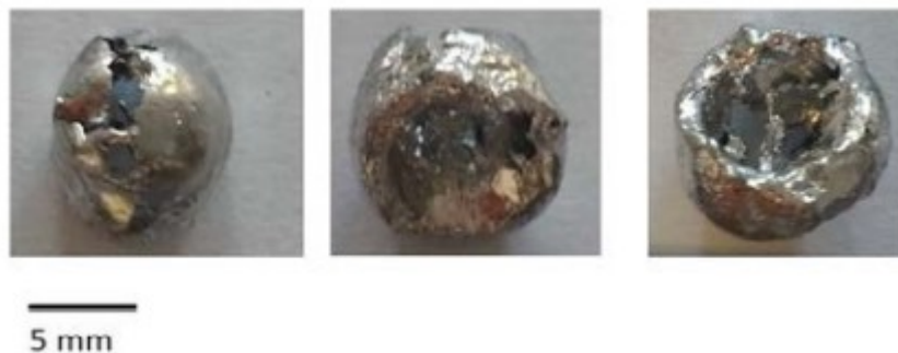
Figure 74: Solidified drop during the formation of forward bag , initial drop of 85 °C and ambient water of 20°C, We = 40 (Achour, 2017)
