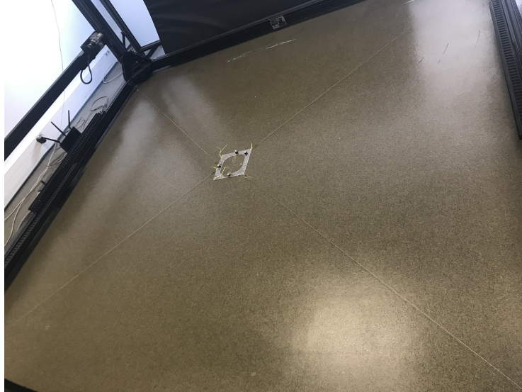
Figure 2.1: The INCA plane robot with 4 cables and platform.
