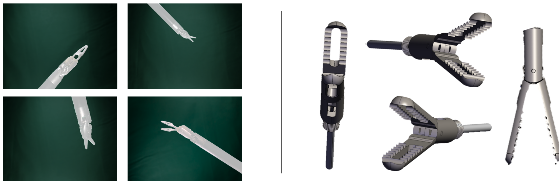
Figure 1.14: Left: shape-priors, in the form of binary segmentation masks of the instruments, obtained from automatic segmentation of chroma-key images. Courtesy of [GPHFD + 21]. Right: different views of a 3D CAD model of a laparoscopic forceps head. Courtesy of [Gra]
