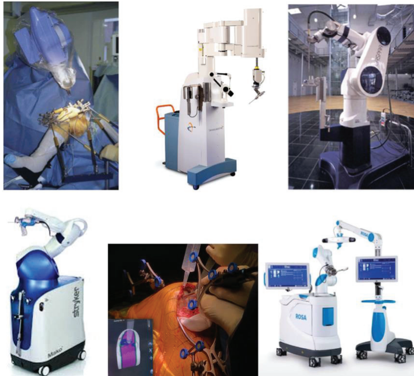
Figure I-4: The autonomous and semiautonomous robotic systems incorporate safeguards against removal of bone beyond the 3D plan. The first three robotic systems are autonomous (Robodoc, Caspar). The last three robotic systems are semiautonomous (Mako, Navio, Rosa).
