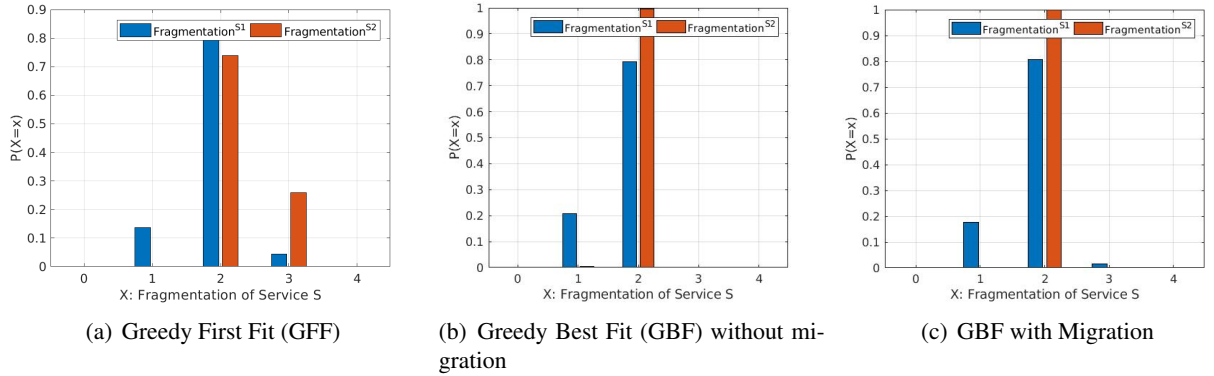
Figure 5.4: Symmetric Cloud topology - Fragmentation of large (in red) versus small (in blue) services
